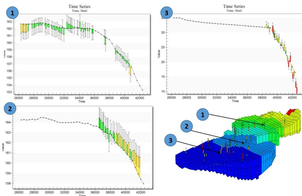
Fig. 6. Observed vs simulated heads in transient state (1971-2016)
