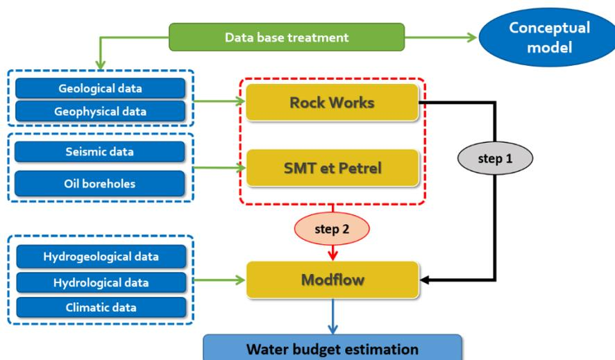
Fig. 3. Adopted methodology for the integration of the 3D geological model into the modflow model
