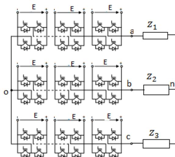
Fig. 1. Example of a three phase multilevel inverter
