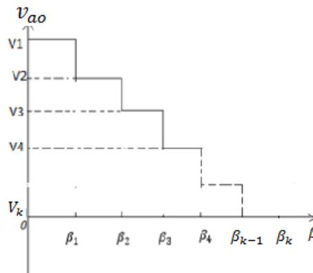
Fig. 2. Phase "a" of a multilevel output signal
