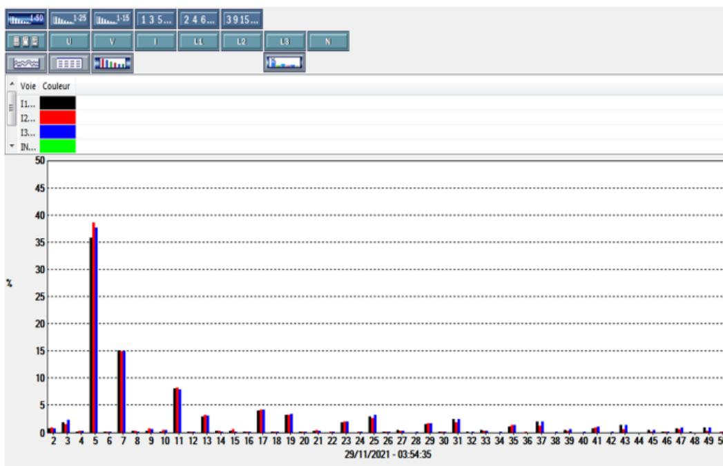
Fig. 3. Current harmonic spectrum of our sample load
