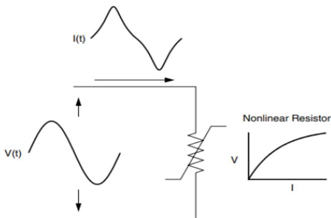
Fig. 1. Current distortion caused by non-linear elements [3]
