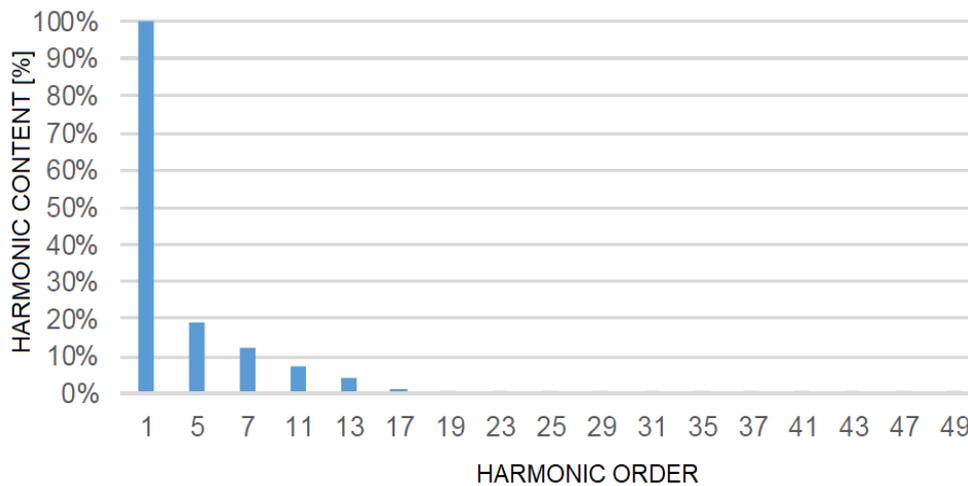
*Fig. 4. Harmonic spectrum for six-pulse FC drives*
