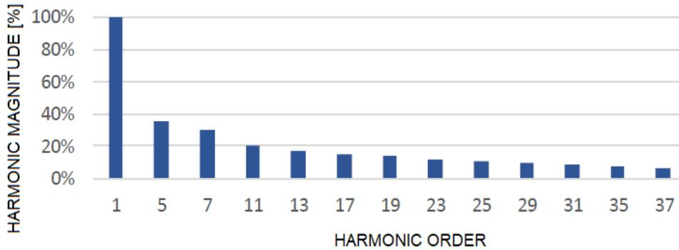
Fig. 2. Characteristic harmonic spectrum - six pulse rectifier
