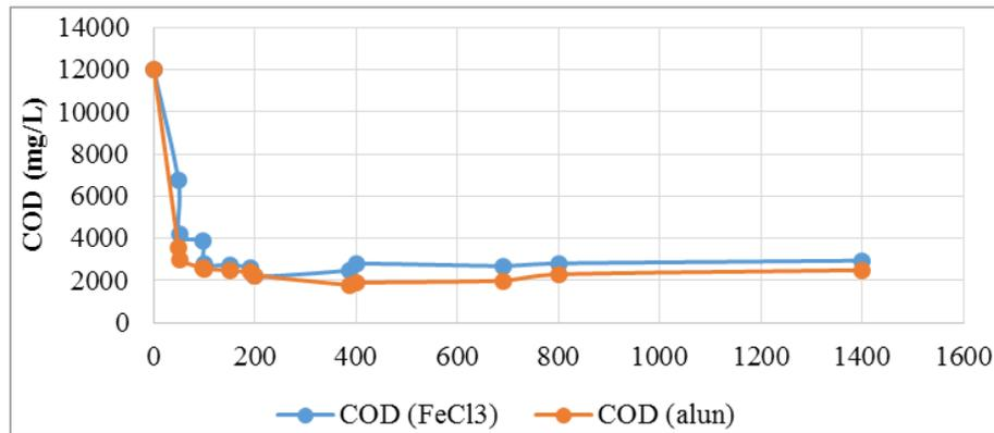
Fig. 1. Effect of coagulant concentration on coagulation-flocculation efficiency.
