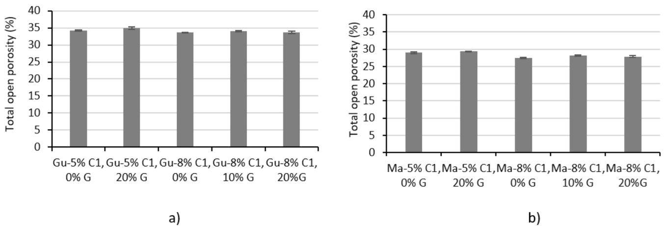
Fig. 8. Effect of decoction on the total open porosity of Gu-based (a) and Ma-based (b) CEB.
