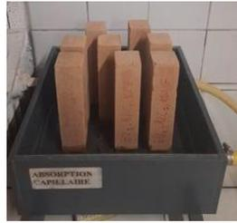
Fig. 4. Capillary water absorption of CEB
