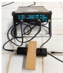
**Fig. 3. Non-destructive dynamic modulus of elasticity method**
