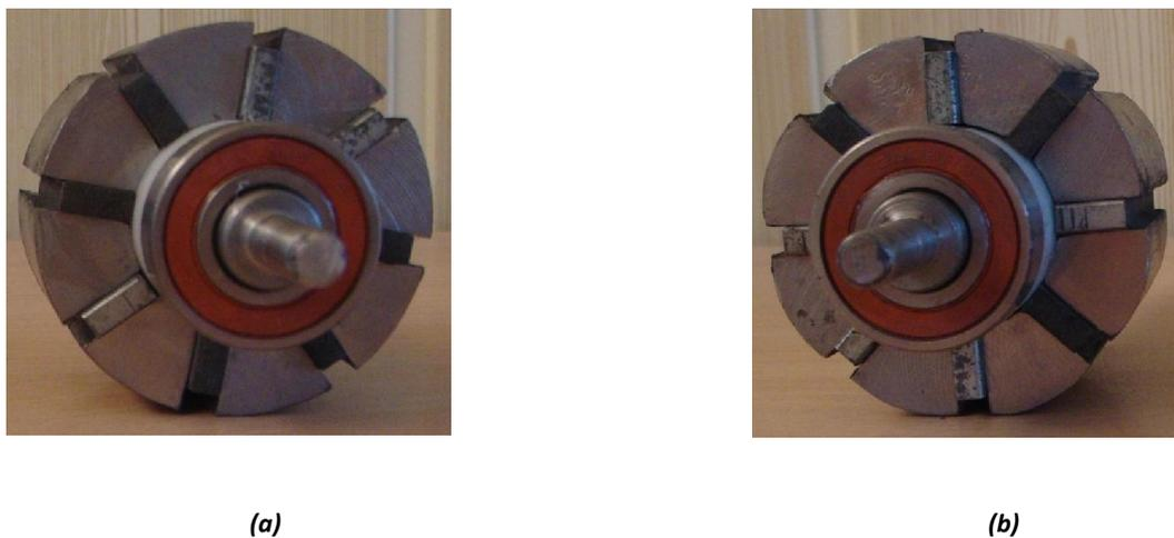
**Fig. 7. The fabricated motors, (a) initial design, (b) optimized design**
