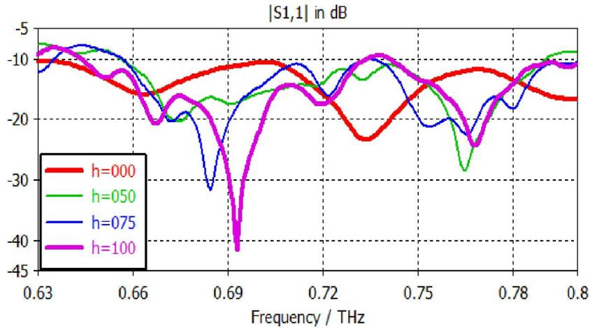
**Fig. 2. Comparison of the reflection coefficient for the structure with and without superstrate. Prototype I:  $h = 0 \text{ }\mu\text{m}$ . Prototype II:  $h = 50 \text{ }\mu\text{m}$ . Prototype III:  $h = 75 \text{ }\mu\text{m}$ . Prototype IV:  $h = 100 \text{ }\mu\text{m}$ .**
