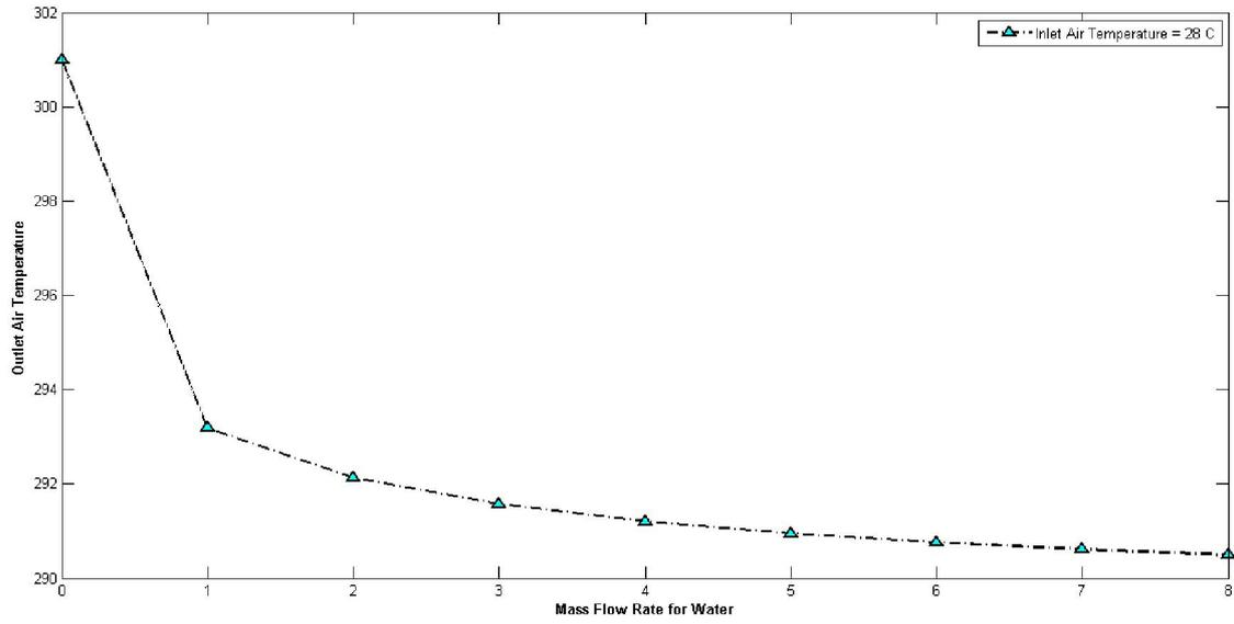
Fig. 5. Outlet air temperature vs mass flow when ambient air temperature is 28 C
