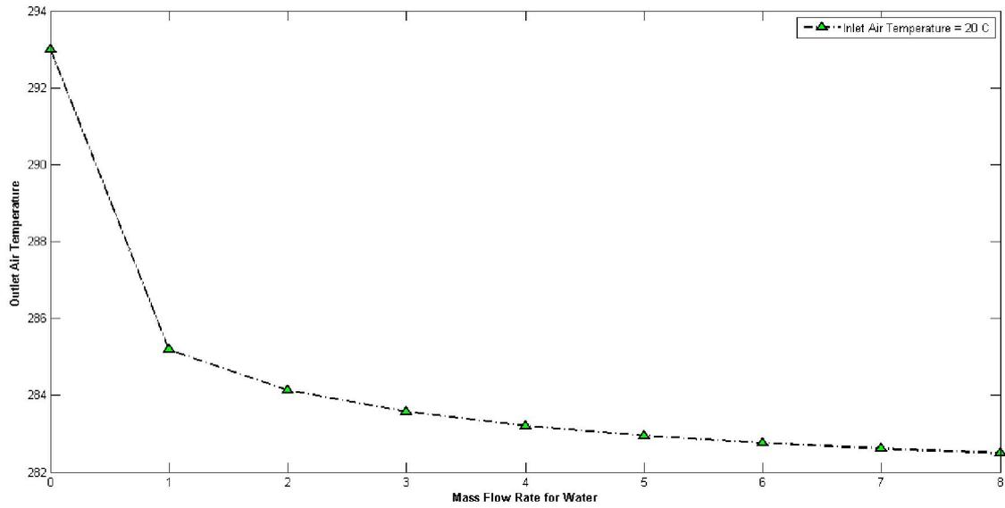
**Fig. 3. Outlet air temperature vs mass flow when ambient air temperature is 20 C**
