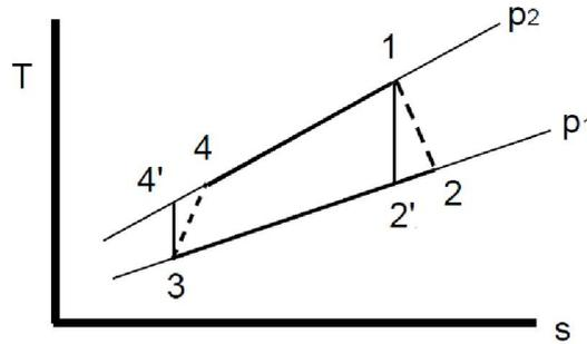
Fig. 1. T-S diagram of gas turbine cycle with combustion at P-constant
