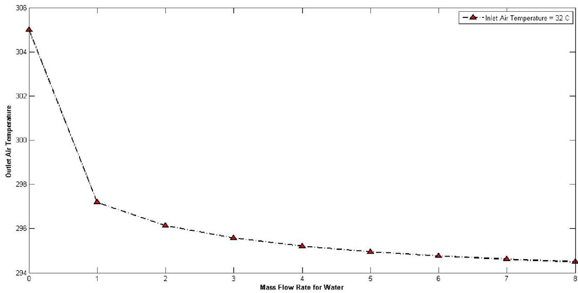
Fig. 6. Outlet air temperature vs mass flow when ambient air temperature is 32 C
