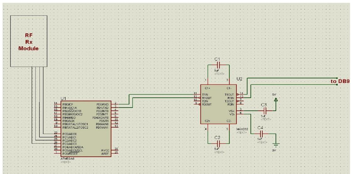
Fig.3: Circuit diagram of an Experimental Work of Receiver side
