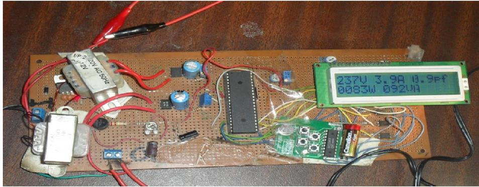
Fig.4: Energy Meter and Transmitter
