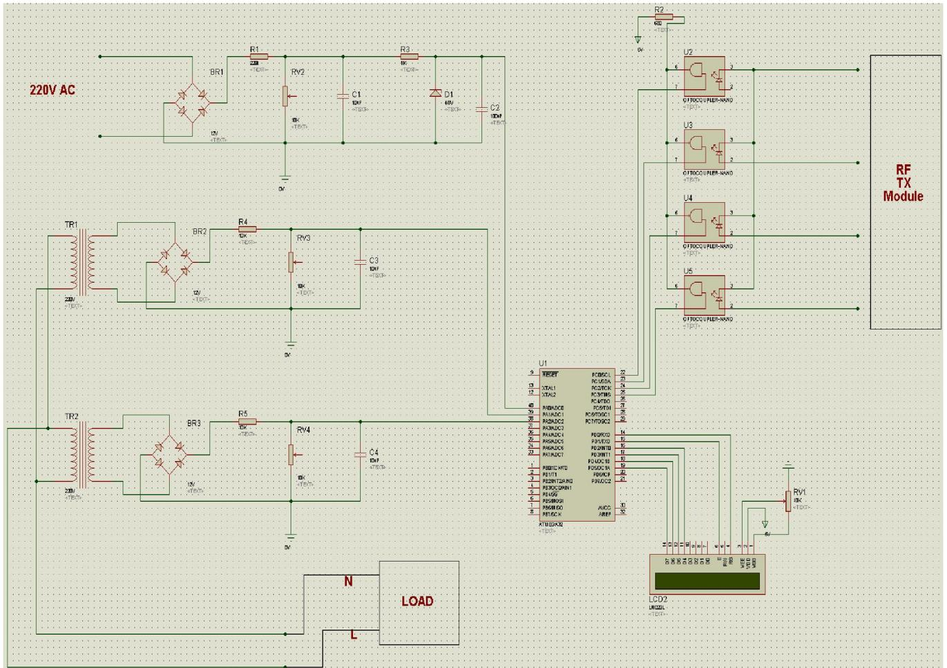
Fig.2: Circuit diagram of an Experimental Work of Energy Meter and Transmitter side
