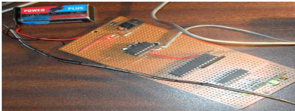
Fig.5: Receiver connected to through serial port to computer
