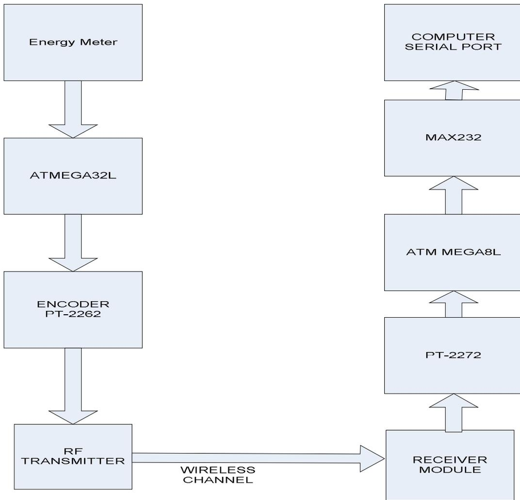
Fig.1 Block Diagram of Experimental Work
