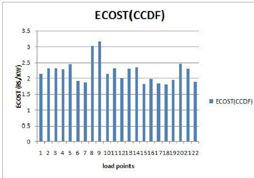
Fig. 3. Calculation of the load point ECOST using the system CCDF
