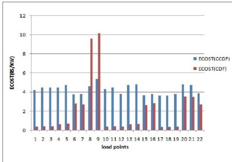
Fig. 5. Comparison of load point ECOST calculated using system CCDF and sector CDF
