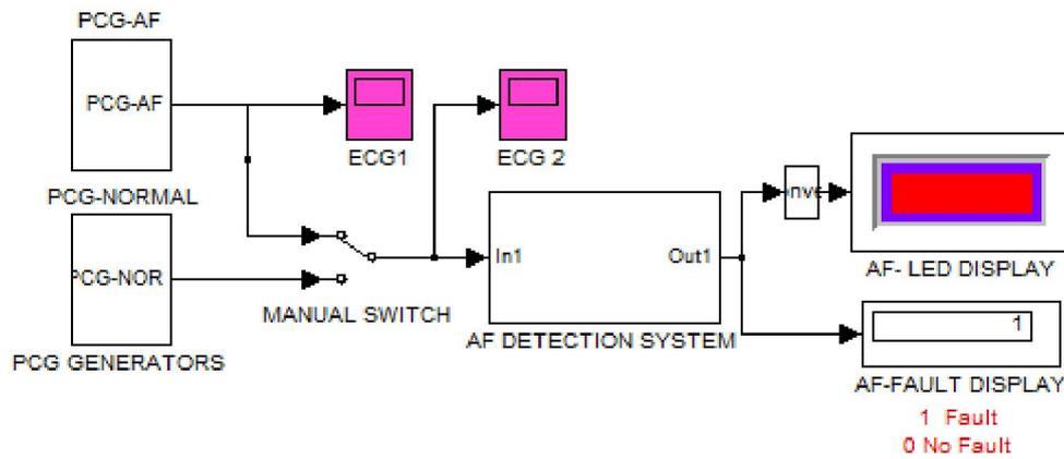
Fig. 6. Simulation of Atrial Fibrillation (AF) heart disease detection
