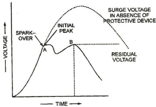
Fig. 1. Voltage Characteristics and Residual Voltage
