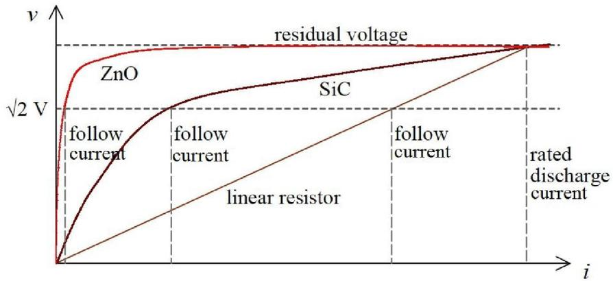
Fig. 3. Volt-Ampere characteristics of non-linear elements
