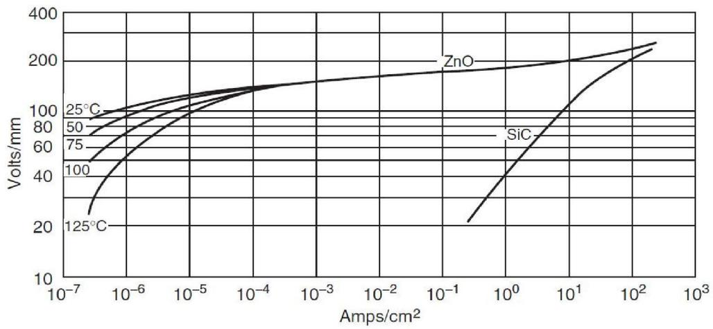
Fig. 4. Volt-Amp characteristics of ZnO and SiC valve element
