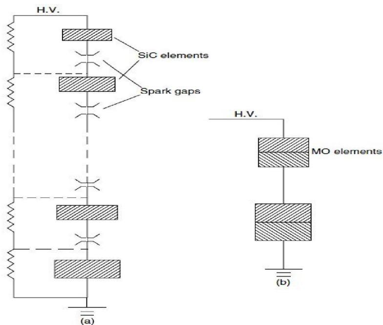
Fig. 2. Block diagram of Silicon Carbide (SiC) and metal oxide arrester (MOA)
