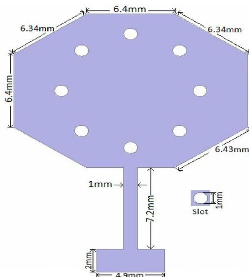
**Fig. 1. Proposed compact microstrip patch antenna**
