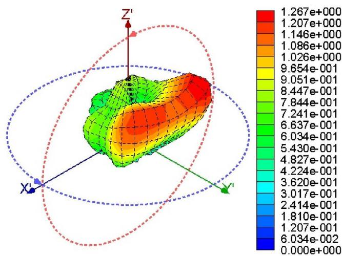
Fig. 8. Far field pattern for 20.10GHz (K-band).
