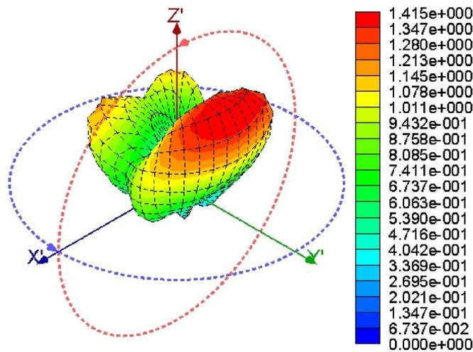
Fig. 7. Far field pattern for 15.70GHz (Ku-band).
