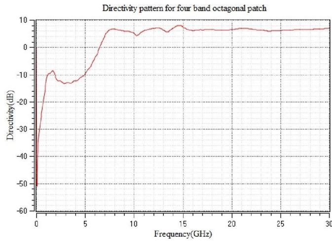
**Fig. 3.** Directivity pattern for octagonal compact patch.
