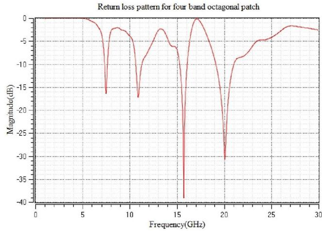
**Fig. 2.** Return loss pattern for octagonal compact patch.
