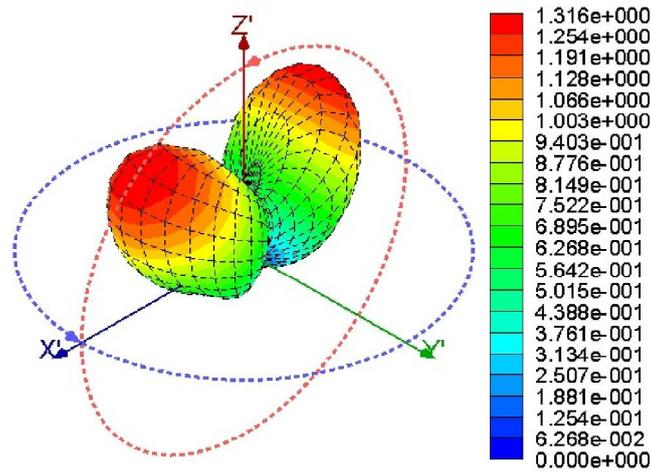
Fig. 6. Far field pattern for 10.89GHz (X-band).
