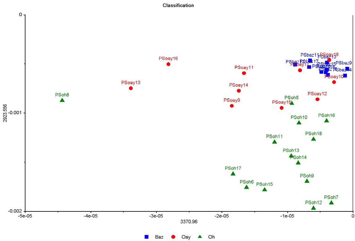
**Fig. 4. 2D score plot of classification results by SVM on calibration. (a) with 2 wavelenths 3370 / 2848  $\text{cm}^{-1}$ ; (b) with 2 wavelenths 3370 / 2923  $\text{cm}^{-1}$**
