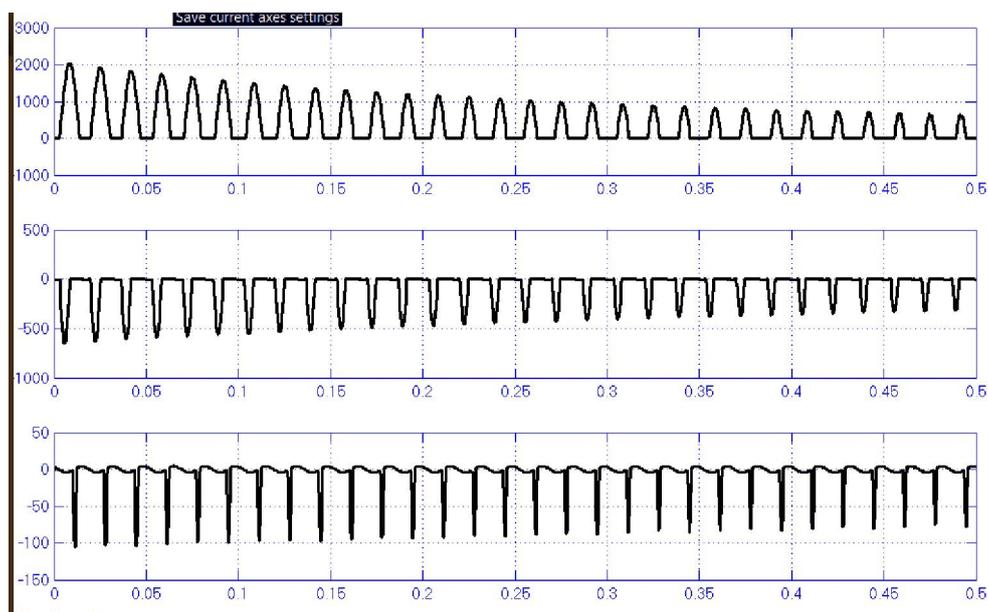
**Fig. 4.** Simulated three phase current waveforms for inrush current
