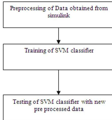
**Fig. 3.** Block diagram of the proposed method for discrimination between magnetic inrush and L-G fault in power transformer
