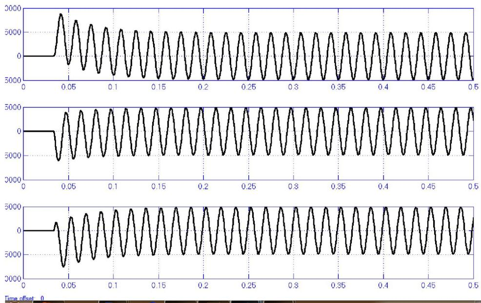
**Fig. 5. Simulated three phase current waveforms for L-G fault current**
