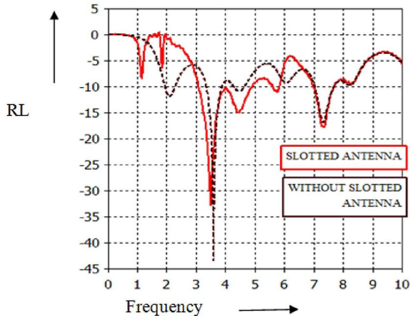
Fig. 2. Return loss against frequency graph
