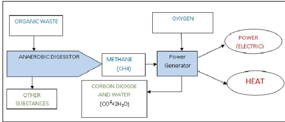
Fig. 9. Schematic diagram of Proposed Biogas production process from organic waste
