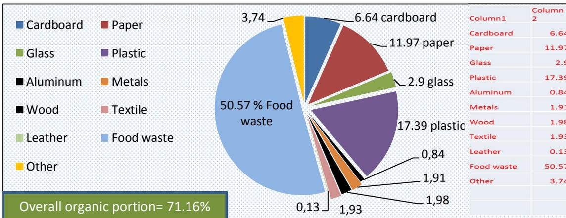
Fig. 5. Composition of overall waste produced in (mass %) KSA
