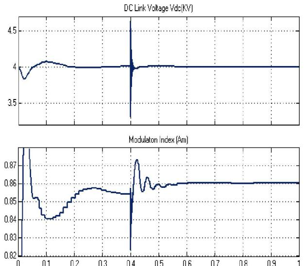
**Fig. 10. DC Link Voltage & Control of Modulation Index**
