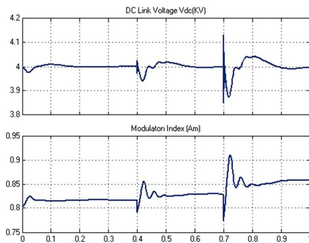
**Fig. 13. DC Link Voltage & Control of Modulation Index**
