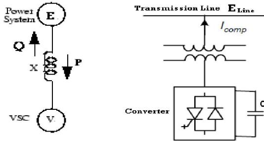
Fig. 1. Static Synchronous Compensator
