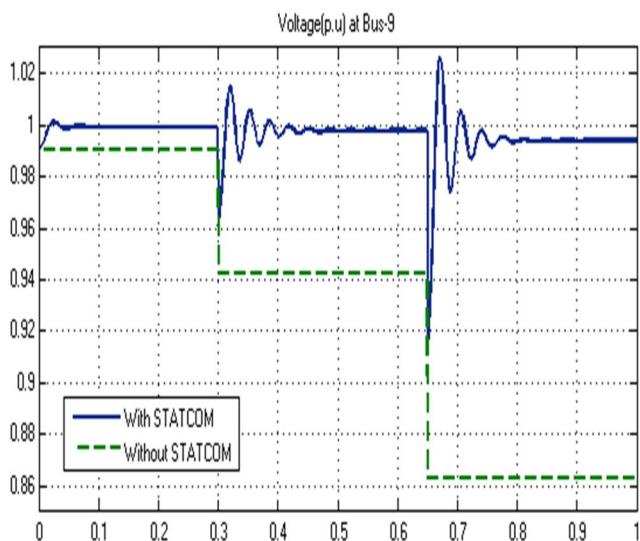
**Fig. 5.** Transmission line voltage at bus-9
