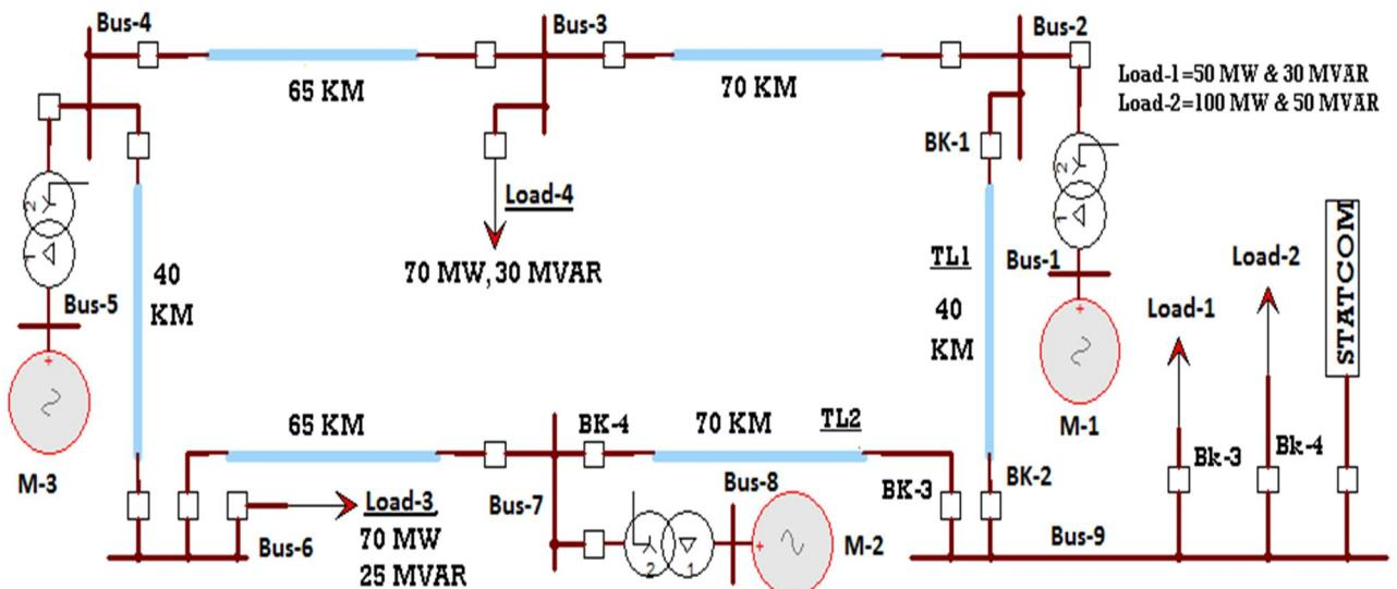
**Fig. 4.** STATCOM connected to the 3 machine 9 bus test System
