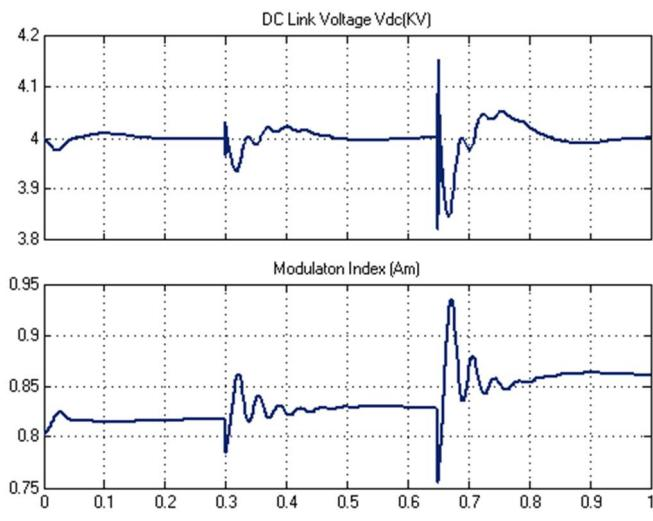
**Fig. 7. DC Link Voltage & Control of Modulation Index**
