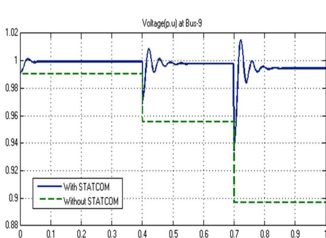
**Fig. 11. Transmission line voltage at bus-9**
