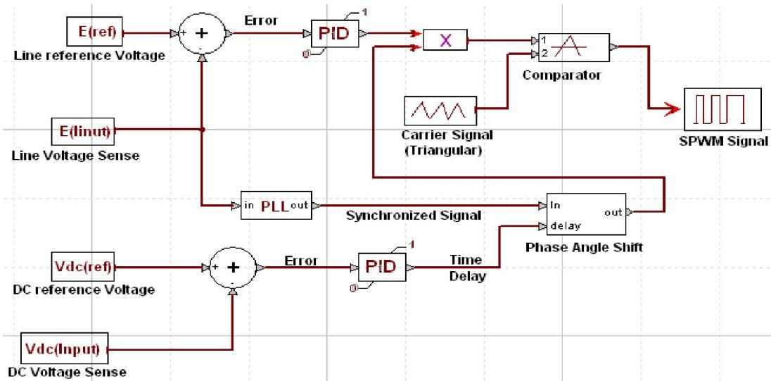
*Fig. 3. Block Diagram of STATCOM Controller*
