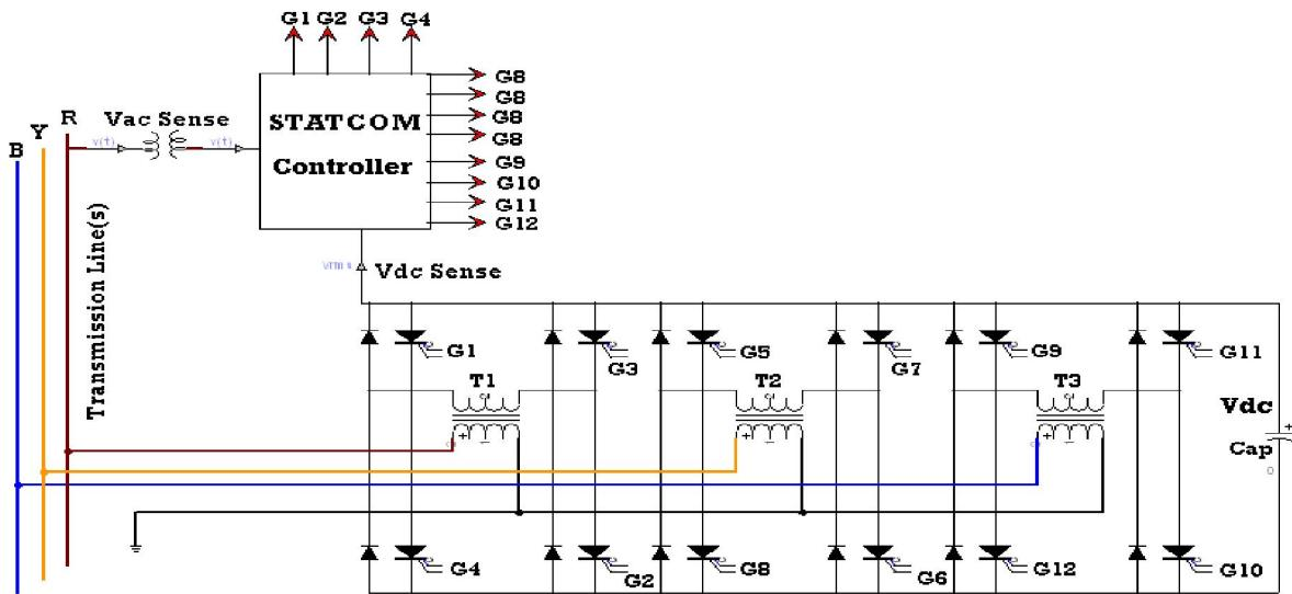
Fig. 2. Modeled Shunt Connected FACTS Device
