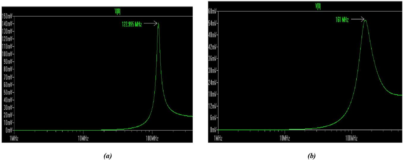
**Fig. 5. (a) Frequency curve of constant Q active inductor bandpass filter with frequency 122.995 MHz and bandwidth is 21 MHz (b) Frequency curve of constant Q active inductor bandpass filter with resistive compensation with frequency 161 MHz and bandwidth is 69.61 MHz**
