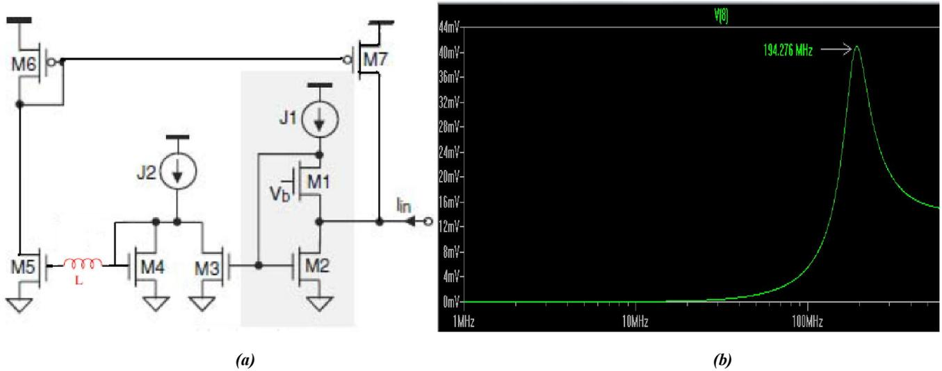
**Fig. 7. (a) Modified constant Q bandpass filter with inductive series peaking (b) frequency response curve with frequency 194.276 MHz and bandwidth is 74.395 MHz**
