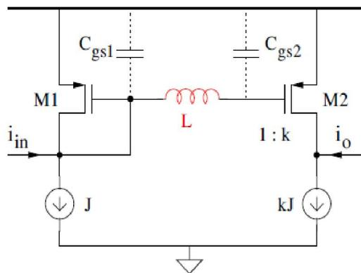
**Fig. 6. Current mirror amplifier with series peaking inductor**
