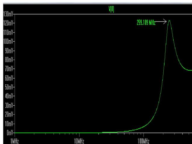
**Fig. 9.** Frequency curve of constant-Q active inductor bandpass filter with inductive series peaking: frequency is 259.189 MHz and bandwidth is 94 MHz
