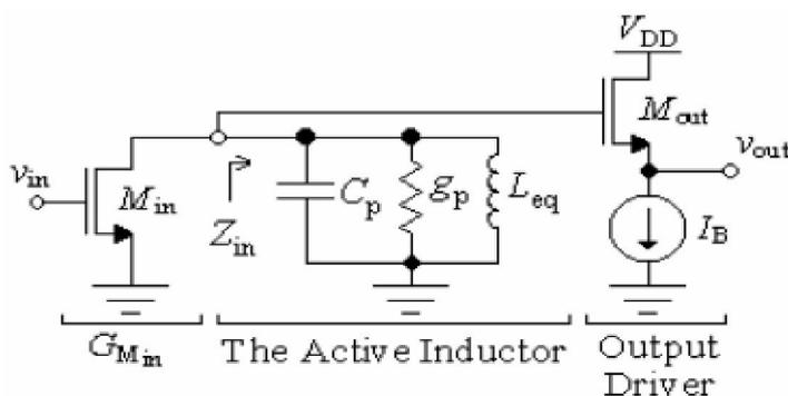
**Fig. 3. Block diagram of the bandpass filter based on active inductor**
