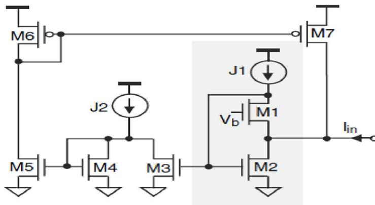
**Fig. 2. Constant-Q CMOS active inductor**
