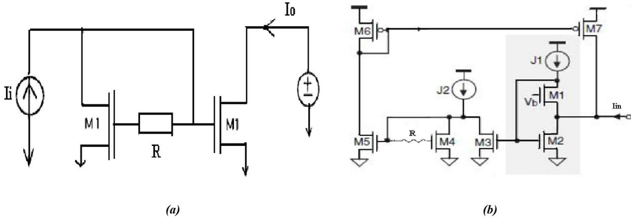
Fig. 4. (a) Simple current mirror (b) Constant-Q active inductor bandpass filter with resistive compensation
