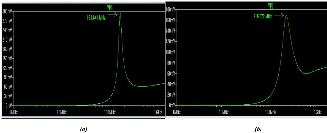
**Fig. 8.** (a) Frequency curve of constant-Q active inductor bandpass filter with frequency is 163.641 MHz and bandwidth is 26 MHz
