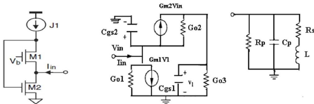
Fig. 1. Wu current reuse active inductor and its equivalent Small signal model and RLC circuit
