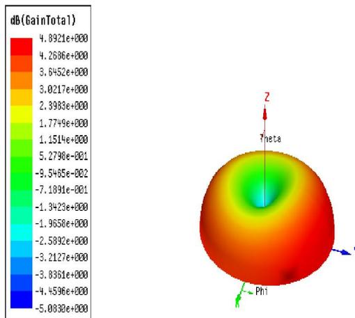
Fig. 9. Gain of an antenna with Metamaterial structure
