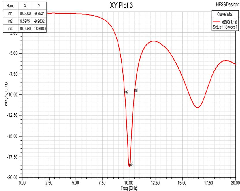
**Fig. 6. Return loss of an antenna without metamaterial structure**
