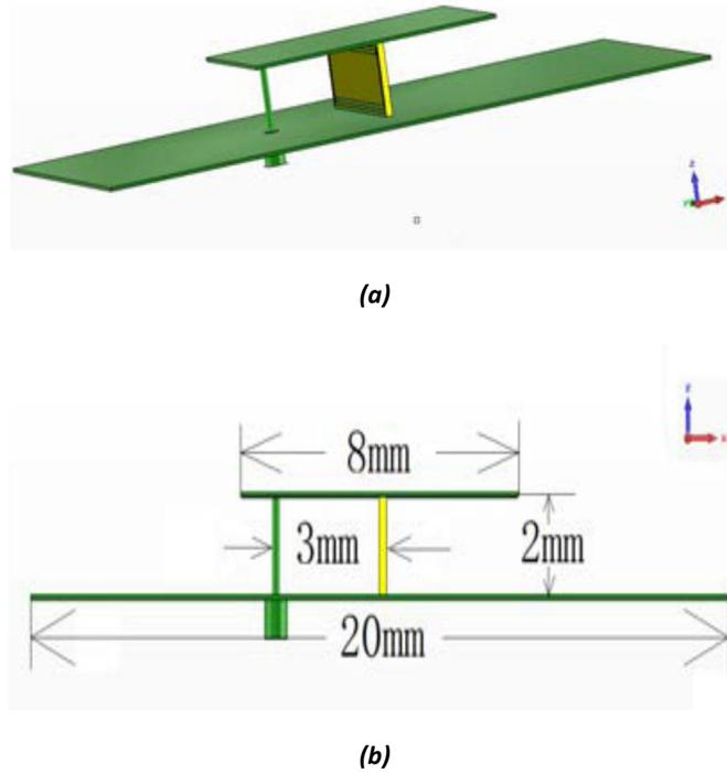
Fig. 3. Sketch of the rectangular patch antenna with the DCR resonator structure, (a) 3D view; (b) xz-plane view
