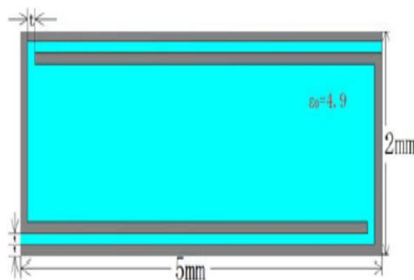
**Fig. 2. Geometry of the rectangular double C shaped structure resonator (DCR)**
