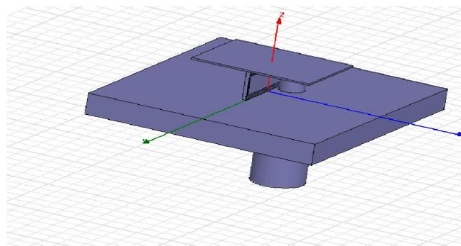
Fig. 4. Rectangular Microstrip antenna with Metamaterial structure
