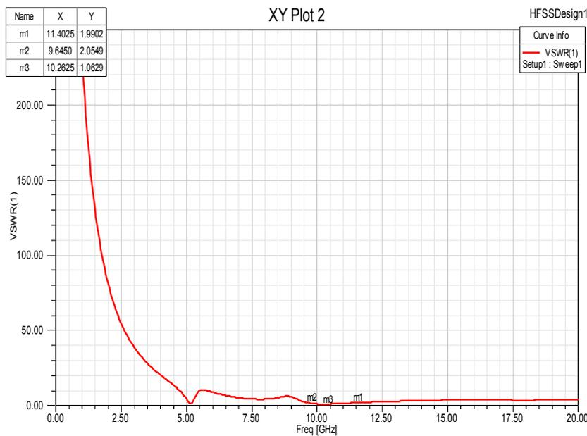
**Fig. 7. VSWR of an antenna with Metamaterial structure**
