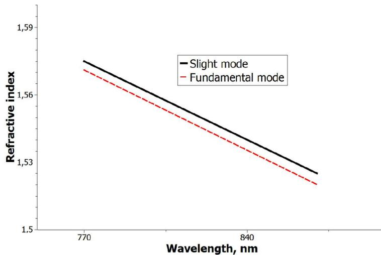
Fig. 3. Dispersion curves of low birefringence PCF (real part of refractive index)
