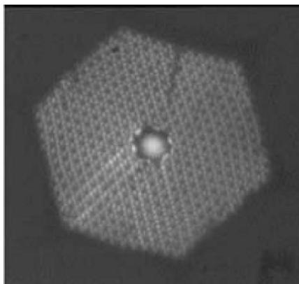
*Fig. 1. Localization of electromagnetic field in photonic crystal fiber [2]*
