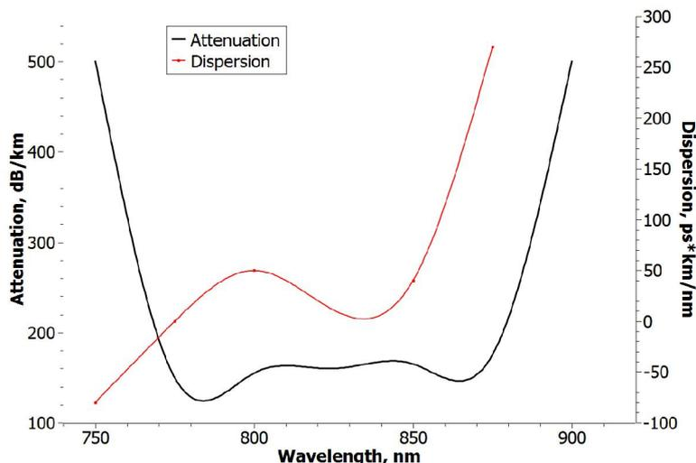
Fig. 5. Dispersion properties of hollow core PCF and its attenuation [6]
