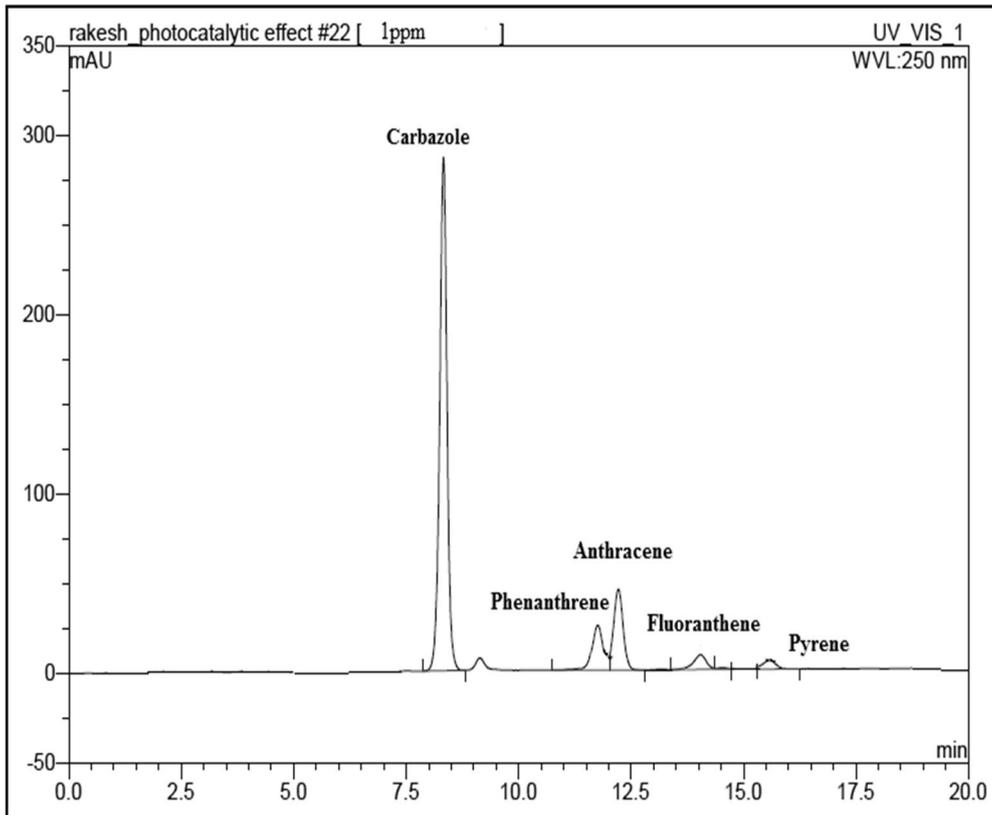
Fig. 2. Standard Chromatogram for HPLC analysis of four PAHs (concentration 1 ppm) and carbazole (20 ppm) with peak height against time
