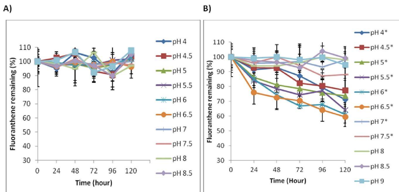
Fig. 7. Percentage fluoranthene remaining in J. Arthur Bower's topsoil at different pH over time exposure to UV light at 375 nm in the presence of  $TiO_2$
