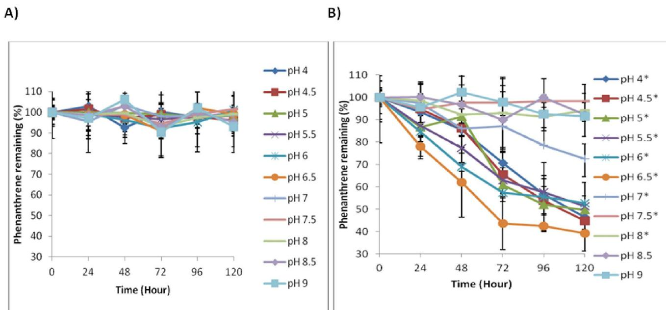
**Fig. 5.** Percentage phenanthrene remaining in J. Arthur Bower's topsoil at different pH over time during exposure to UV light at 375 nm in the presence of  $TiO_2$
