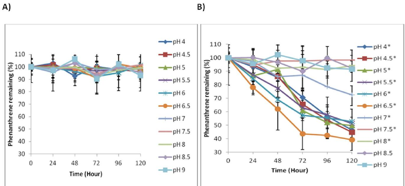
**Fig. 5.** Percentage phenanthrene remaining in J. Arthur Bower's topsoil at different pH over time during exposure to UV light at 375 nm in the presence of  $\text{TiO}_2$
