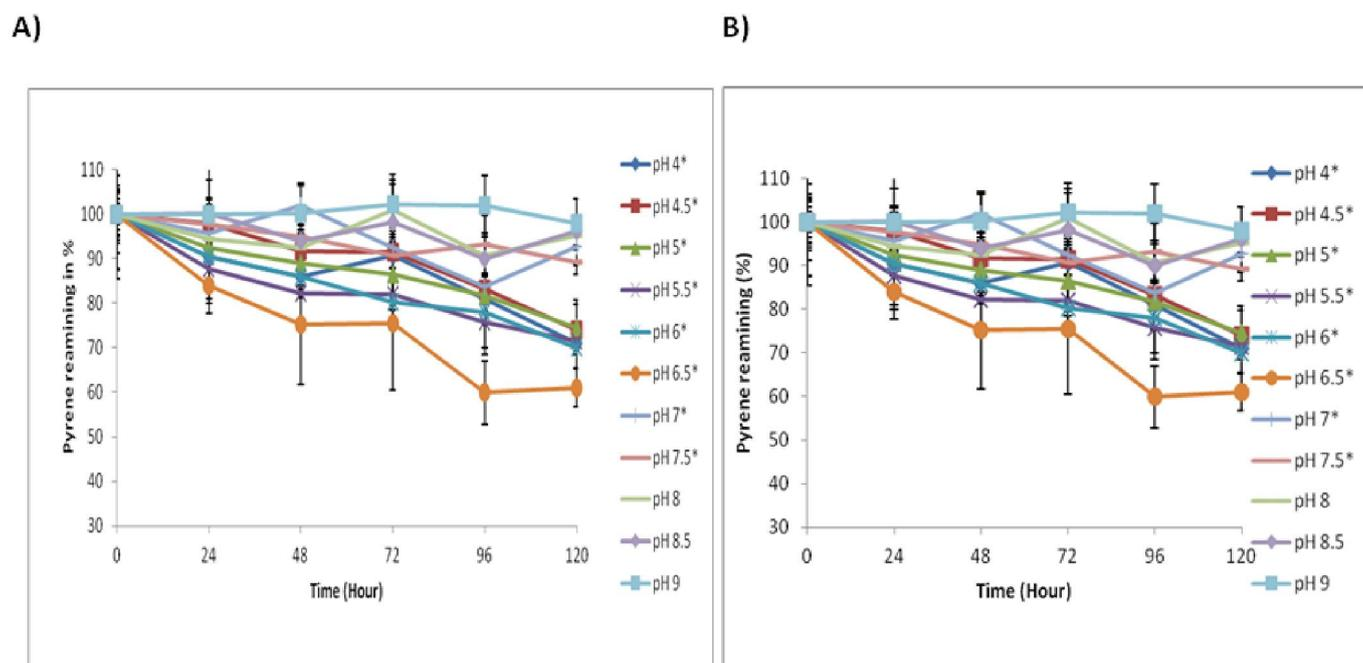
**Fig. 12.** Percentage pyrene remaining in J. Arthur Bower's topsoil at different pH over time during exposure to UV light at 254 nm in the presence of  $\text{TiO}_2$
