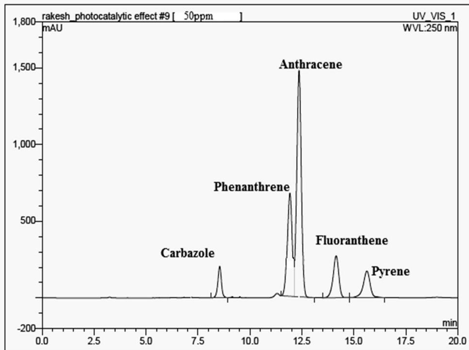
Fig. 3. Standard chromatogram for HPLC analysis of four PAHs (concentration 50 ppm) and carbazole (20 ppm) with peak height against time
