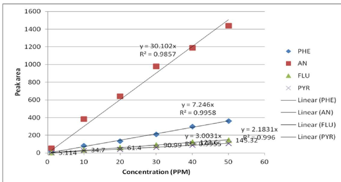
Fig. 4. HPLC standard curve of four PAH showing peak area against concentration. PAH used and their symbol abbreviations are (PHE) Phenanthrene; (AN) Anthracene; (FLU) Fluoranthene; (PYR) Pyrene
