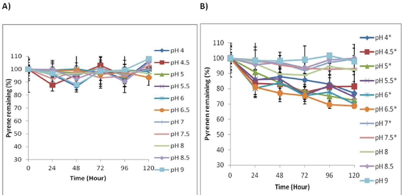
**Fig. 8.** Percentage pyrene remaining in J. Arthur Bower's topsoil at different pH over time during exposure to UV light at 375 nm in the presence of TiO<sub>2</sub>
