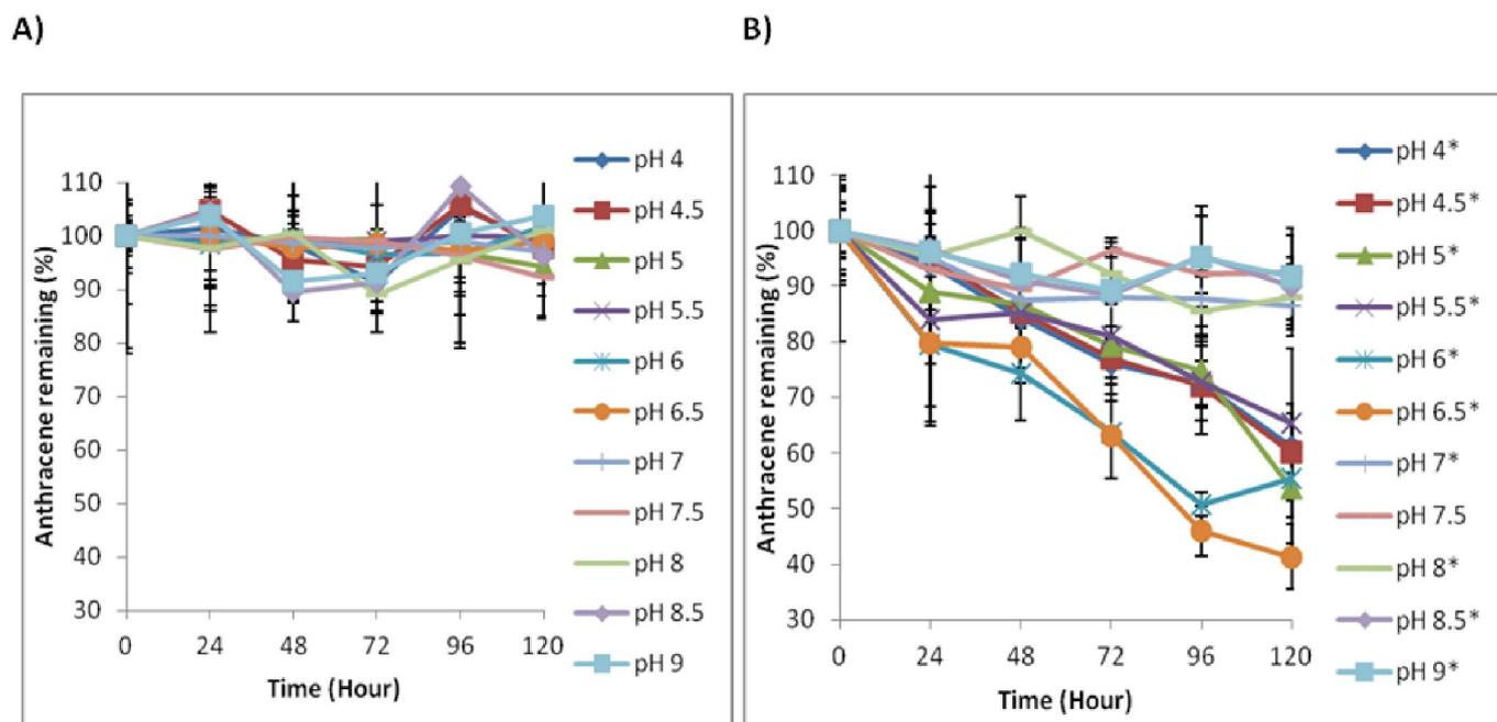
**Fig. 6.** Percentage anthracene remaining in *J. Arthur Bower's* topsoil at different pH over time during exposure to UV light at 375 nm in the presence of  $TiO_2$
