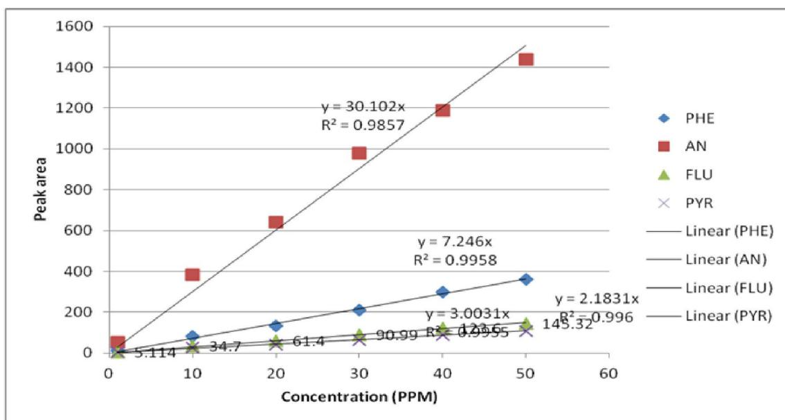
Fig. 4. HPLC standard curve of four PAH showing peak area against concentration. PAH used and their symbol abbreviations are (PHE) Phenanthrene; (AN) Anthracene; (FLU) Fluoranthene; (PYR) Pyrene
