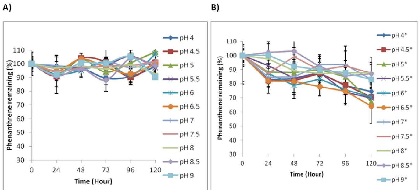
**Fig. 9.** Percentage phenanthrene remaining in J. Arthur Bower's topsoil at different pH over time during exposure to UV light at 254 nm in the presence of TiO<sub>2</sub>
