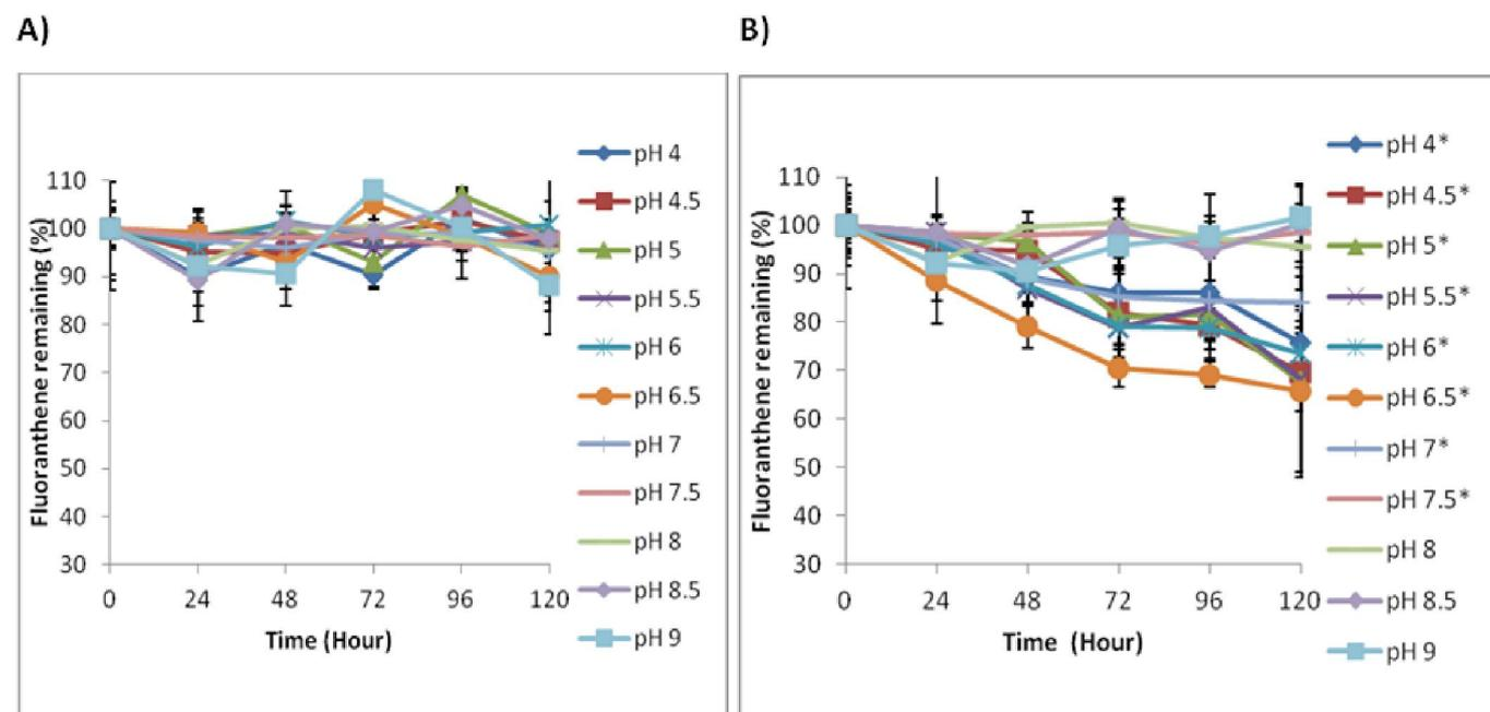
**Fig. 11. Percentage fluoranthene remaining in J. Arthur Bower's topsoil at different pH over time during exposure to UV light 254 nm in the presence of TiO<sub>2</sub>**
