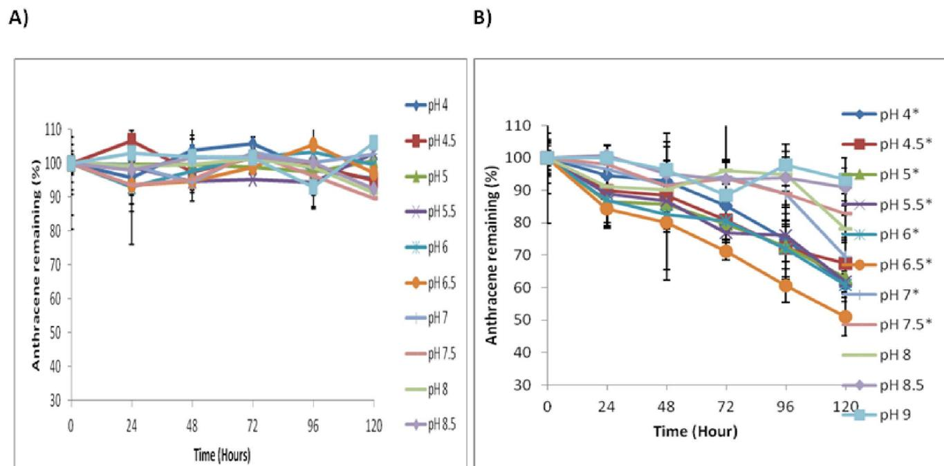
Fig. 10. Percentage anthracene remaining in J. Arthur Bower's topsoil at different pH over time during exposure to UV light 254 nm in the presence of TiO<sub>2</sub>
