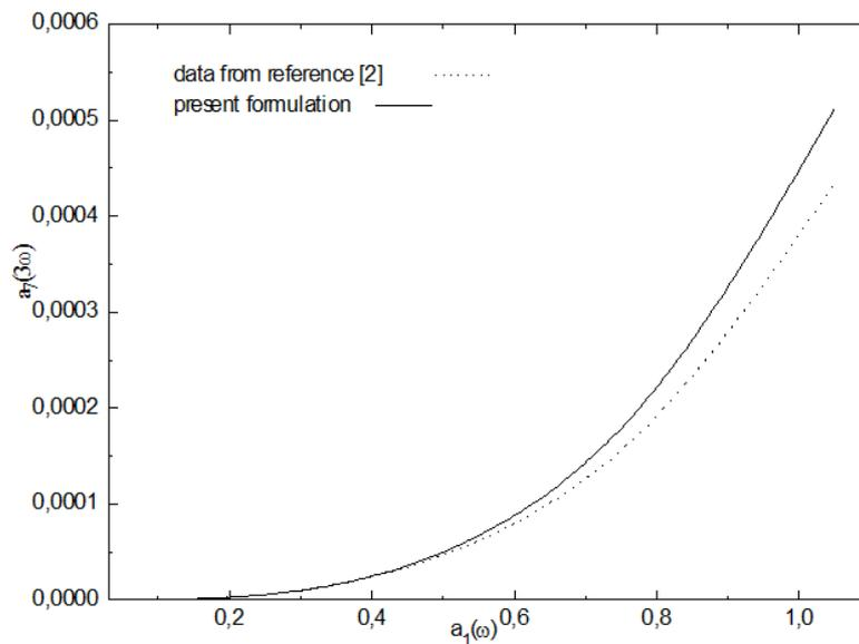
**Fig. 4. Comparison between the contribution  $a_7(3\omega)$  of the data taken from reference [2] and the present formulation of the C-C beam**
