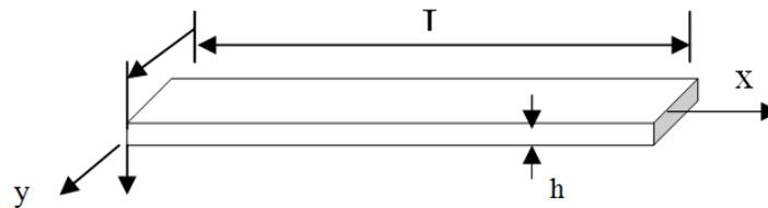
**Fig. 1. Co-ordinates system for the beam**
