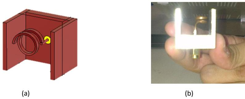
Fig. 1. Design of Pi-wall partial cavity backed 1½ turn helical antenna
