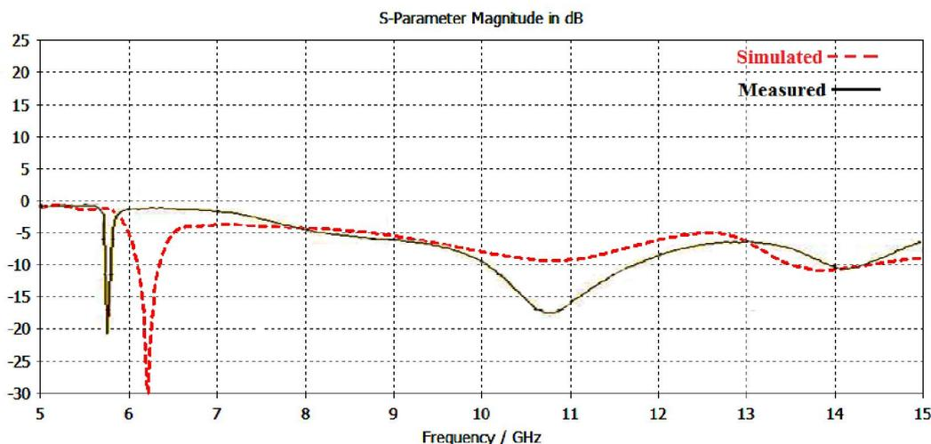
**Fig. 7.** Plot of reflection coefficient at  $315^\circ$  helix rotation
