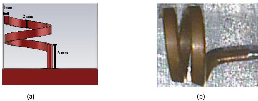
Fig. 2. Helix geometrical configuration
