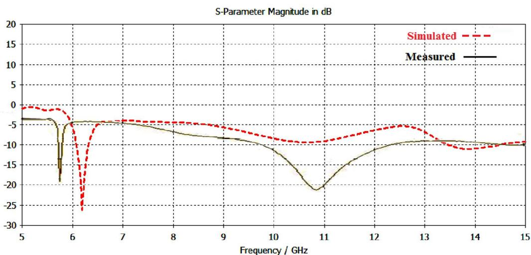
Fig. 6. Plot of reflection coefficient at 135° helix rotation
