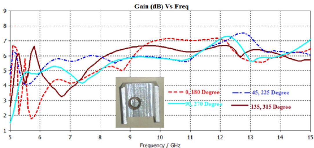
Fig. 5. Comparative gain plot at various helix rotation angles
