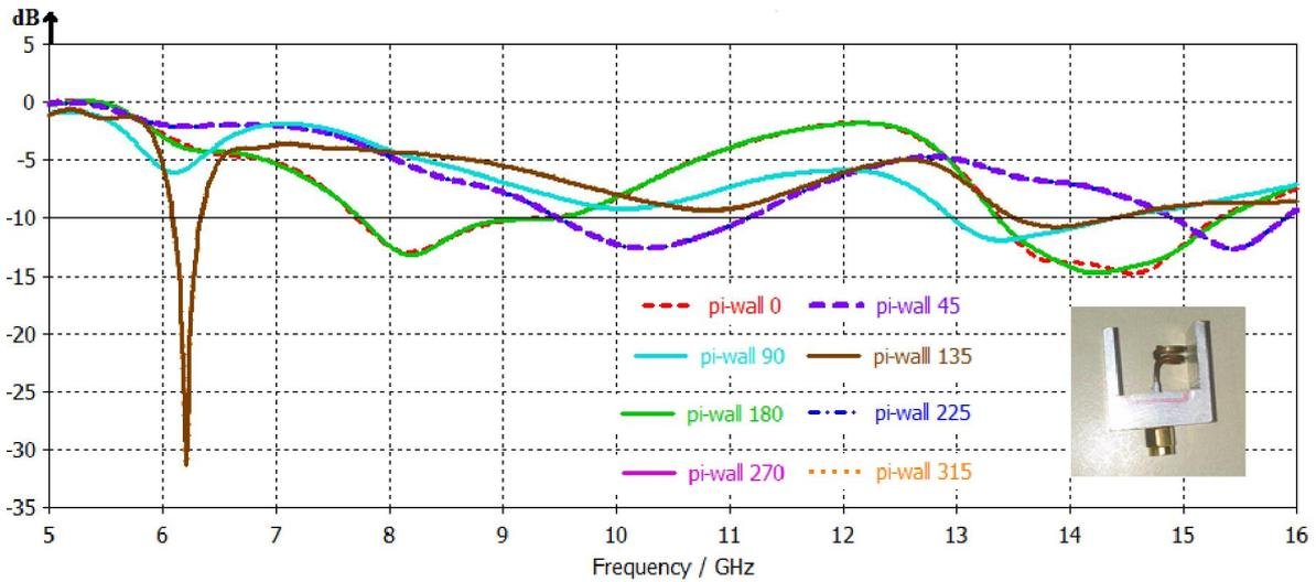
**Fig. 4. Comparative plot of reflection coefficient at various helix rotations**
