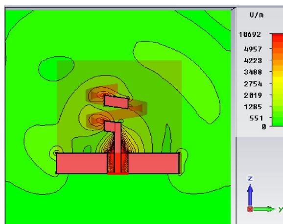
**Fig. 8.** Near E-field distribution in Pi-wall cavity
