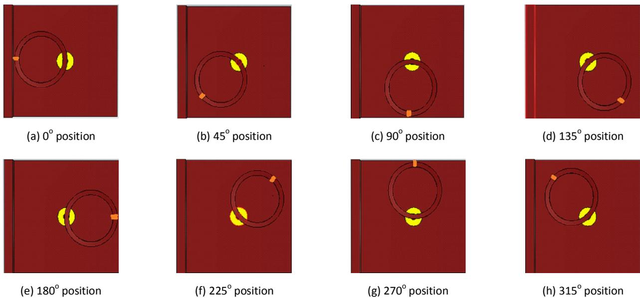
Fig. 3. Top view of helix rotation inside the Pi-wall shaped cavity
