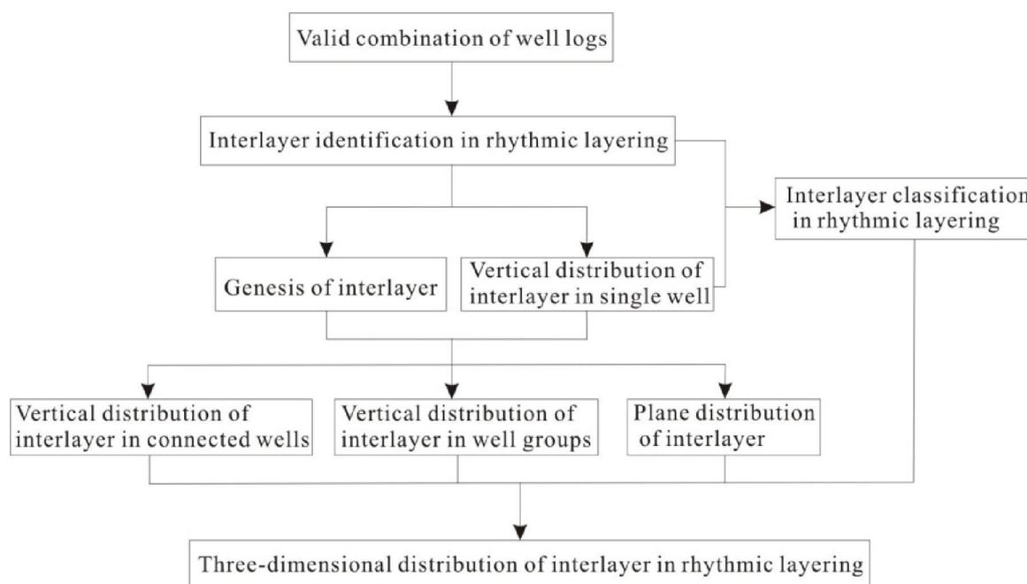
**Fig. 1. Flow diagram showing a comprehensive characterization method of interlayer in rhythmic layering**
