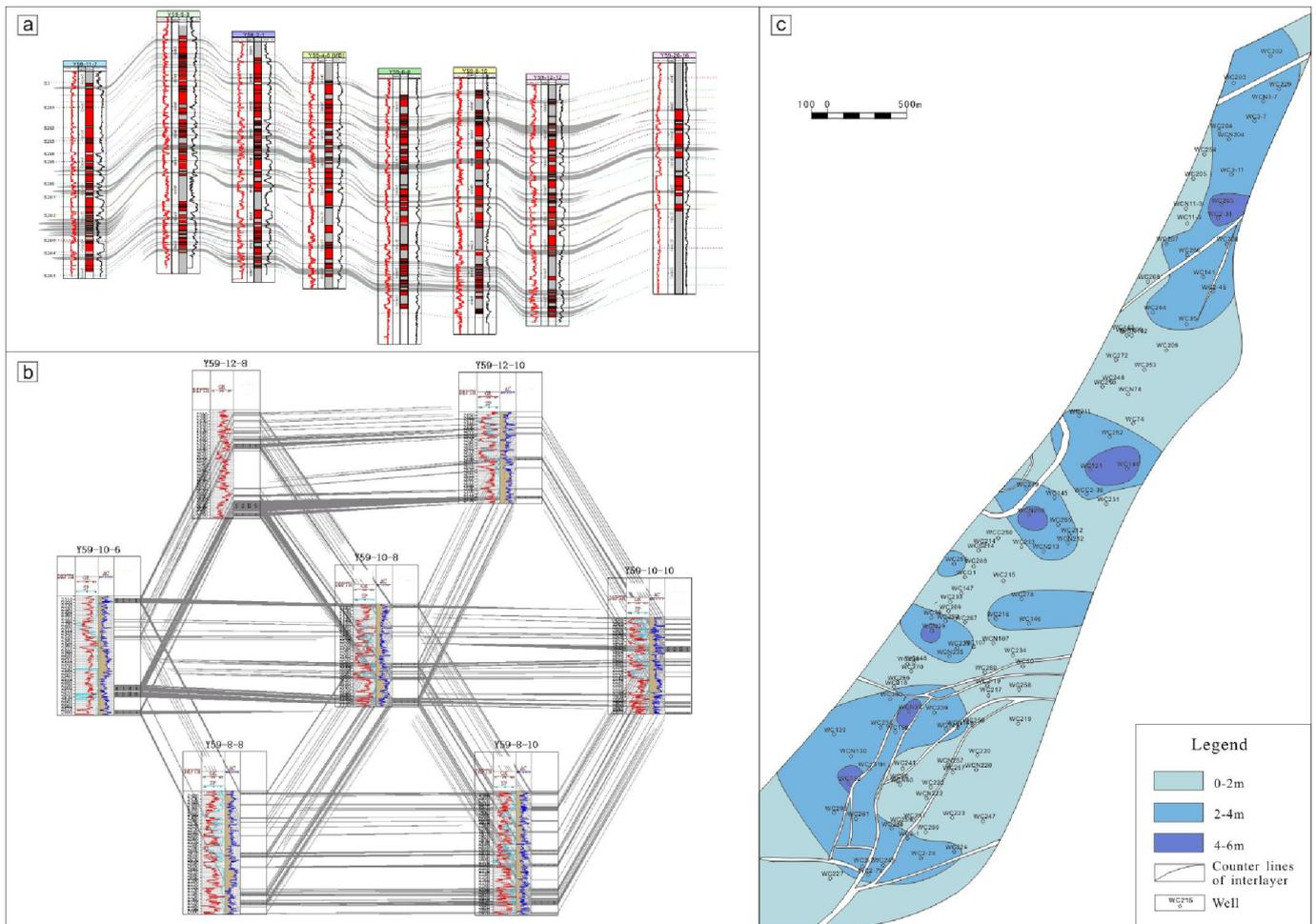
**Fig. 3. Map showing the distribution characteristics of interlayer plotted on cross-well sections, well group, and plane**
