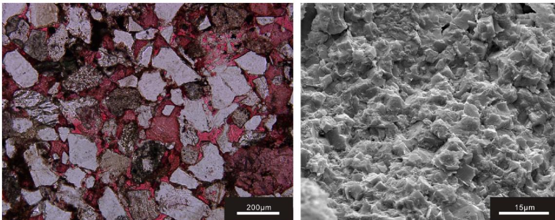
**Fig. 2. Thin section and scanning electron photomicrographs showing calcareous cement contents of calcium interlayer**
