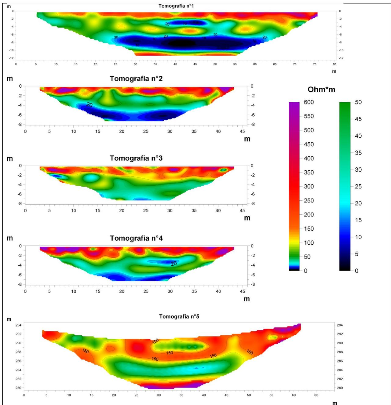
Fig. 2. Resistivity model for the Ovar landfill with contaminated areas
