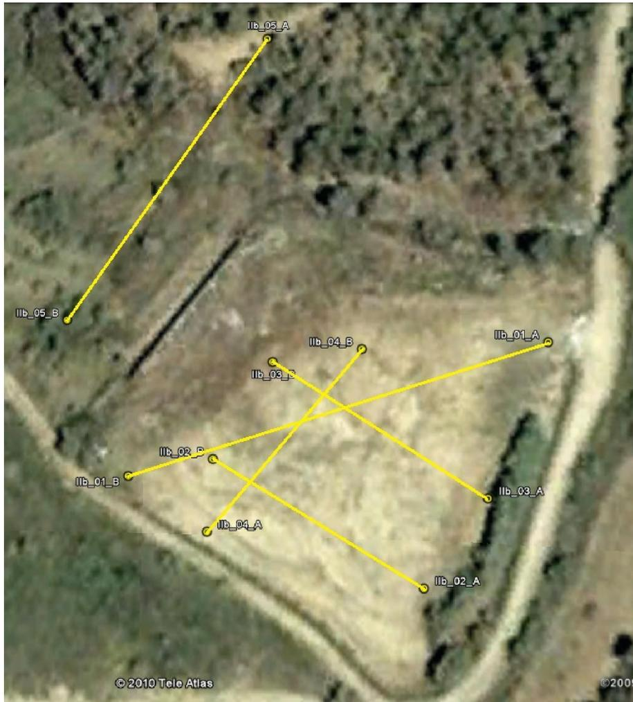
**Fig. 1. Aerial photography of the landfill with the positioning of the ERT profiles**
