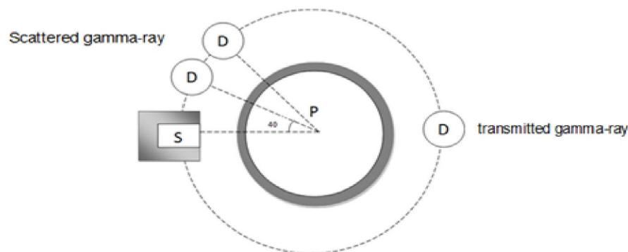
Fig. 1. Different configuration setups of density measurement system.
