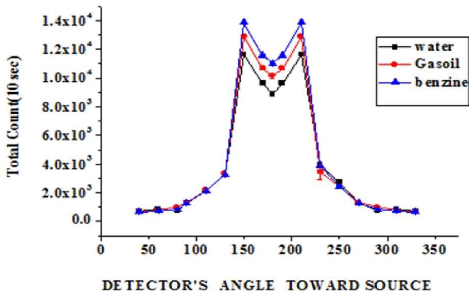
Fig. 5. Count rate versus detector angle for PVC pipe (Experiment)
