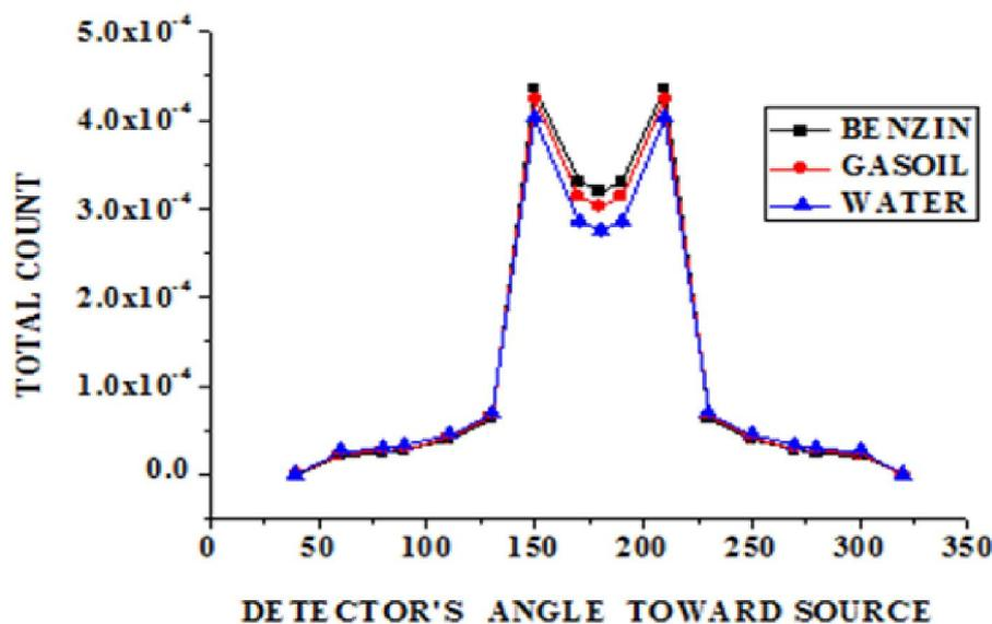
Fig. 3. Count rate vs. detector angle for PVC pipe (MCNP simulation)
