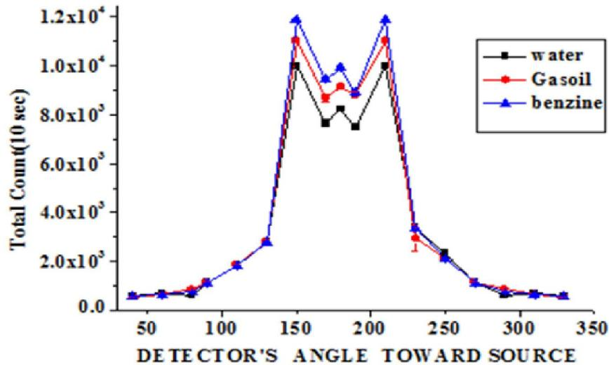
Fig. 4. Count rate versus detector angle for iron pipe (Experiment)
