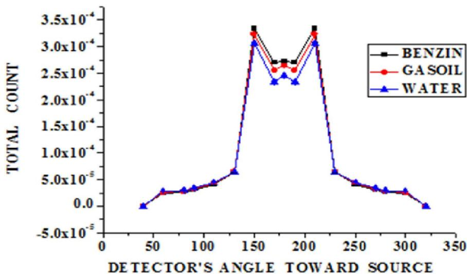
Fig. 2. Count rate vs. detector angle for iron pipe (MCNP simulation)
