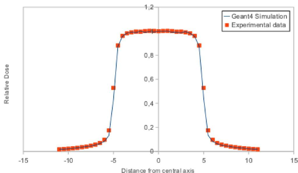
Fig. 7. Comparison of calculated and measured dose profile at the depth of 10 cm due to 12 MV photon beam in homogeneous water phantom, for a  $10 \times 10 \text{ cm}^2$  field size
