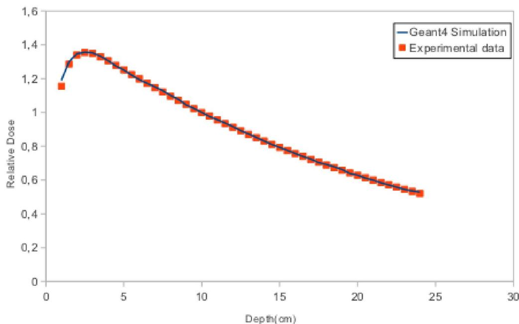
**Fig. 8.** Comparison of calculated and experimental relative depth dose due to 12 MV photon beam in homogeneous water phantom, for a  $10 \times 10 \text{ cm}^2$  field size. Results are normalized to the dose at the depth of 10 cm
