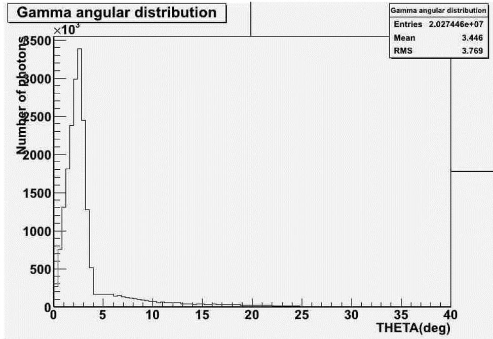
Fig. 3. Gamma angular distribution below Jaws (SSD 50cm)
