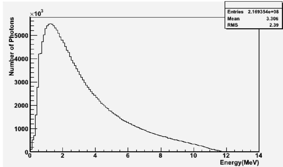
Fig. 6. Monte Carlo calculated spectrum photon energy spectrum at SSD 90 cm for 12 MV photon beam
