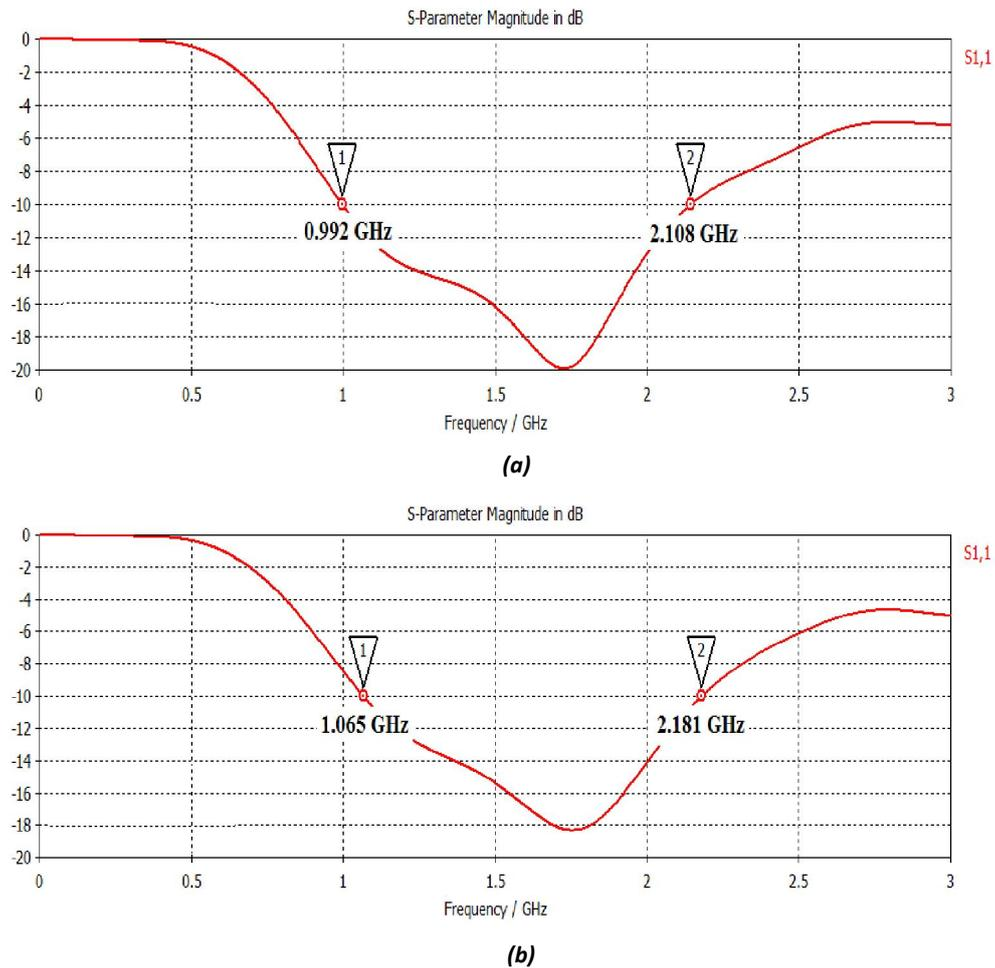
**Fig. 6. Simulated return loss for (a) PRMA-1 (b) PRMA-2**
