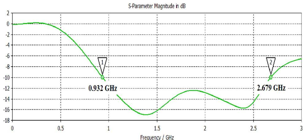
**Fig. 8. Simulated result of the proposed PHMA**
