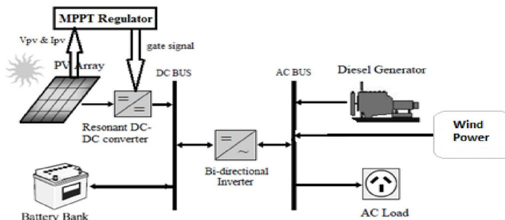
Fig. 1. Block diagram for parallel configuration of hybrid systems
