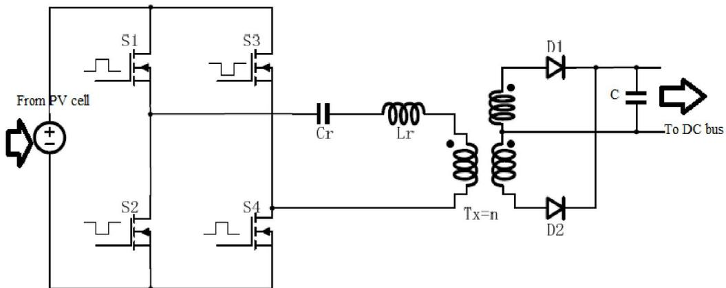
Fig. 5. Circuit diagram of Hybrid Bridge DC- DC converter
