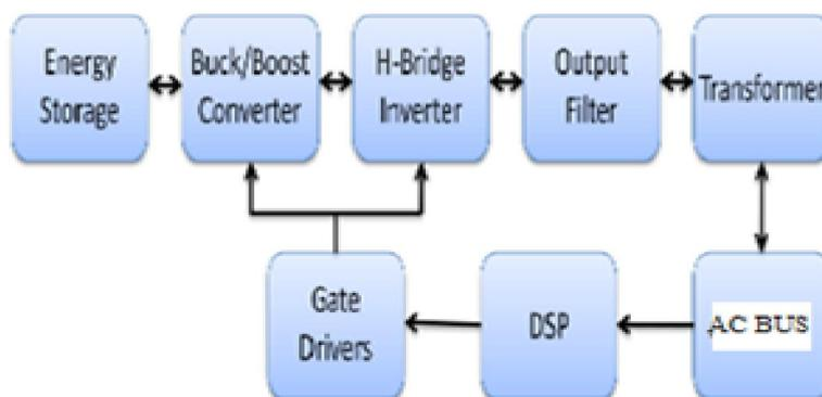
**Fig. 7. Bi-directional Inverter block diagram**
