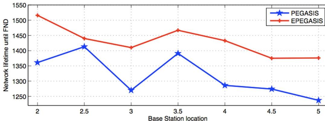
Fig. 4. Network lifetime vs Base station location
