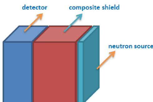
Fig. 1. Simulation geometry in order to find the optimal amount of boron in the safeguard [12]
