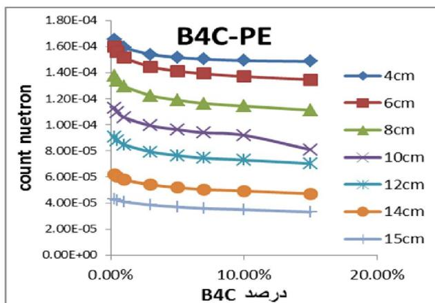
Fig. 2. Neutron's count changes due to adding boron to the safeguard's different thicknesses [19]
