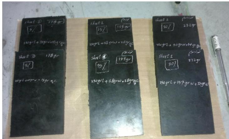
Fig. 3. Three examples of elastic safeguard made with boron carbide and tungsten impurity
