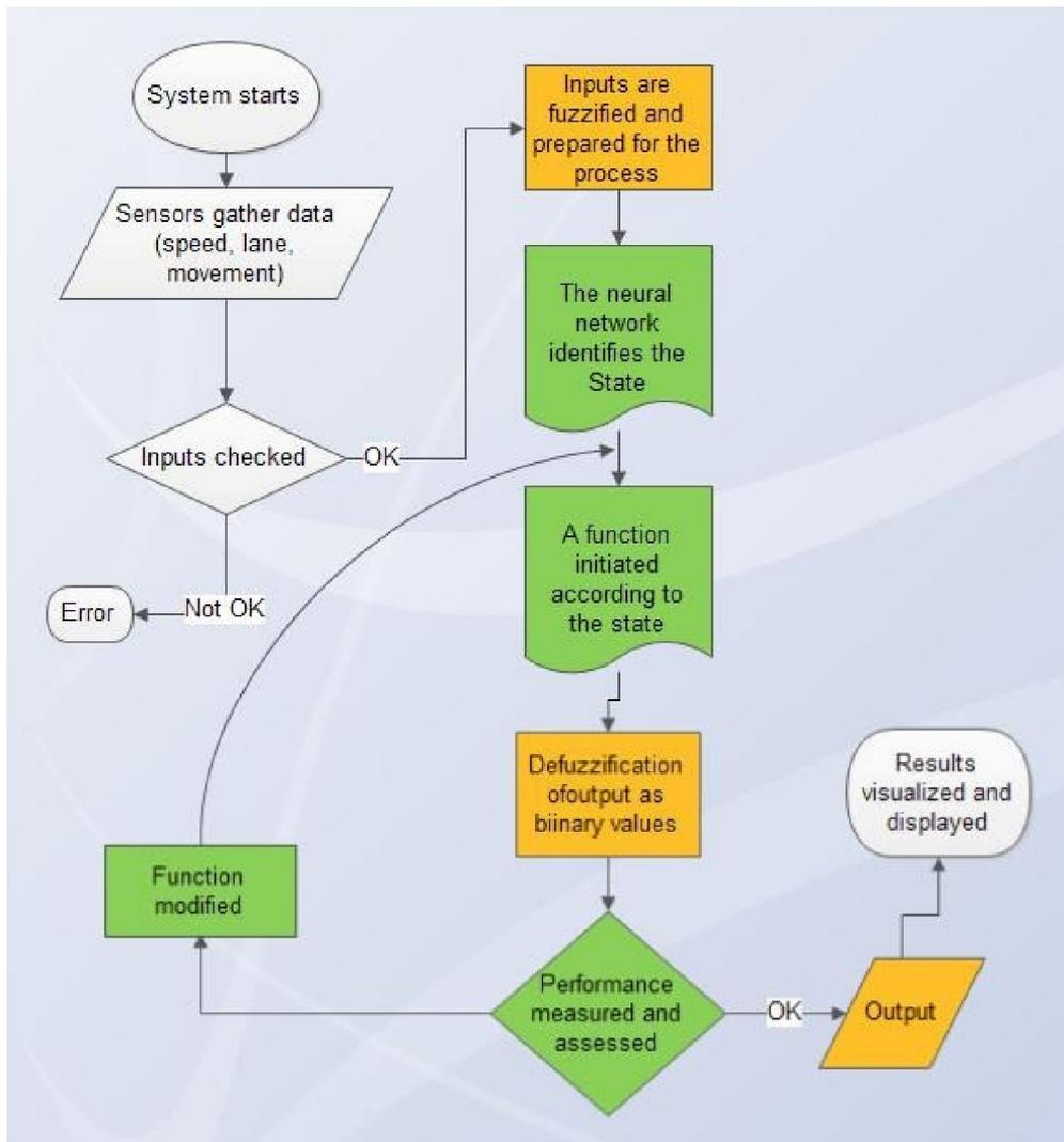
**Fig. 4.** The whole process flowchart (Green objects form the Neuro part of the process and the orange objects the Fuzzy aspect of the process)
