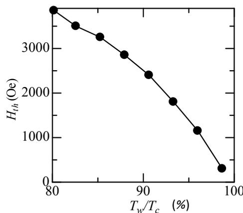
Fig. 4. The profile of threshold field towards the temperature on  $K_I = 4.5 \times 10^5 \text{ erg/cm}^3$ ,  $4\pi M_s = 2100 \text{ G}$ , and  $T_w = 298.0 - 372.9 \text{ K}$
