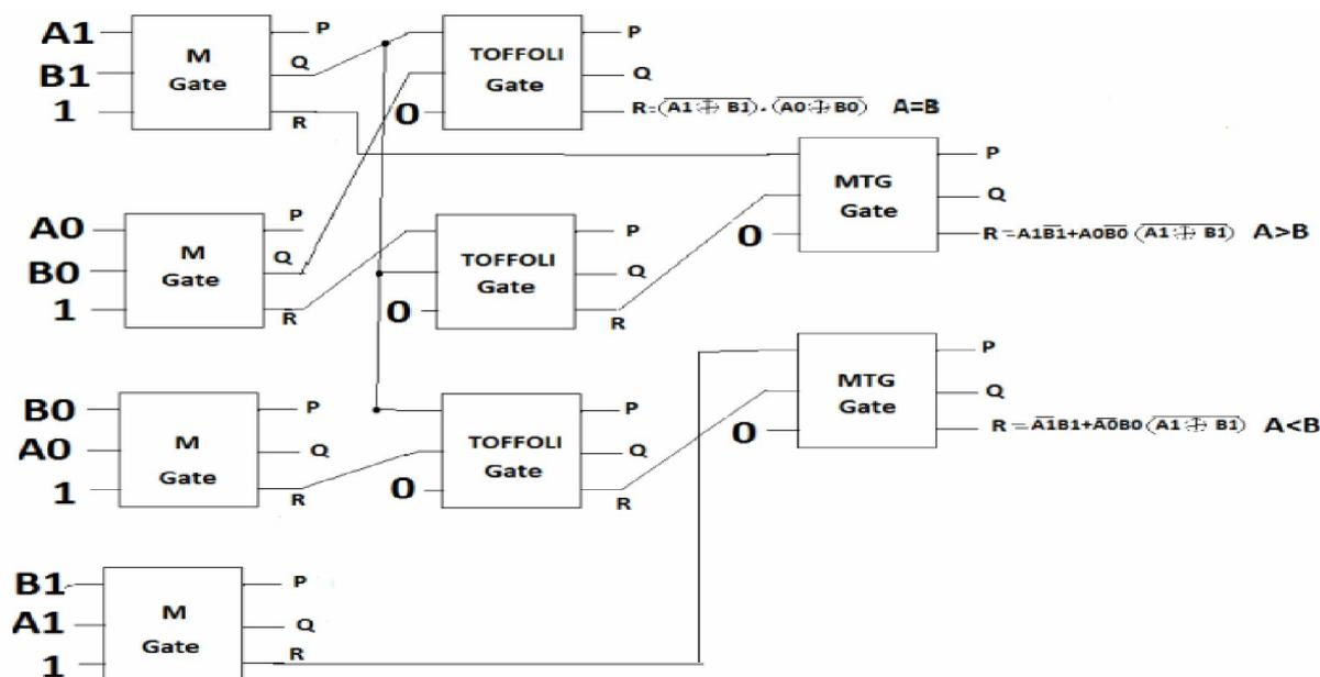
Fig. 4. Architecture for Reversible 2 bit Comparator unit
