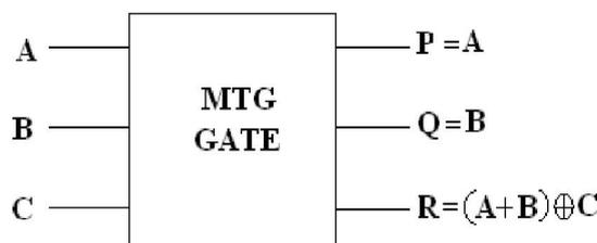
Fig. 3. Reversible logic MTG gate
