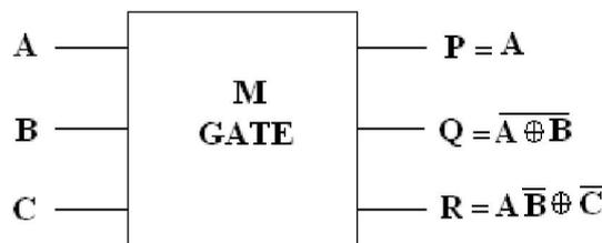
Fig. 2. Reversible logic M gate
