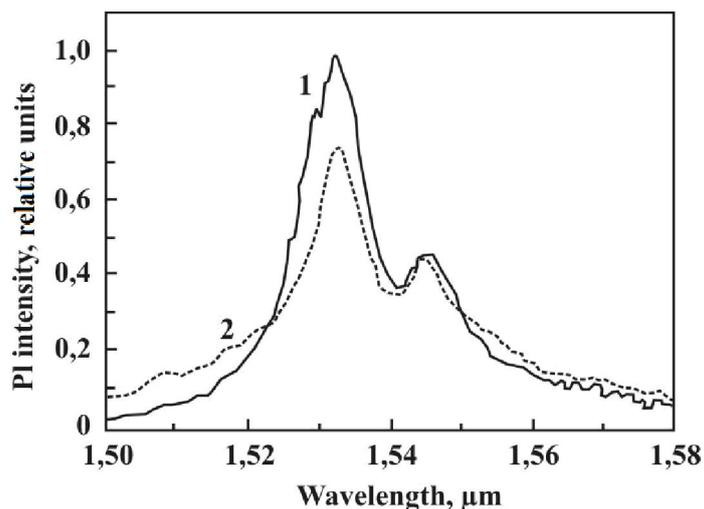
**Fig. 3.** Spectral characteristic of a film ( $Er_2O_3 - SiO_x - Al_2O_3$ ) on the fragment of optical fiber
