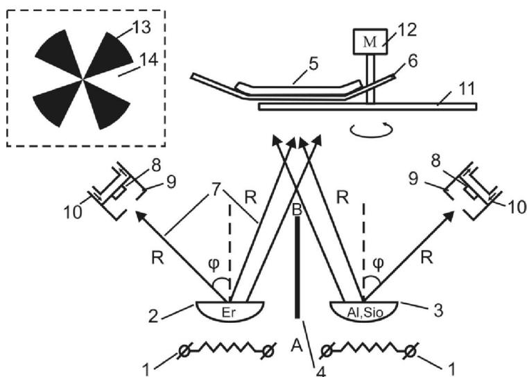
**Fig. 1. Equipment for vacuum controllable deposition of multicomponent films**
