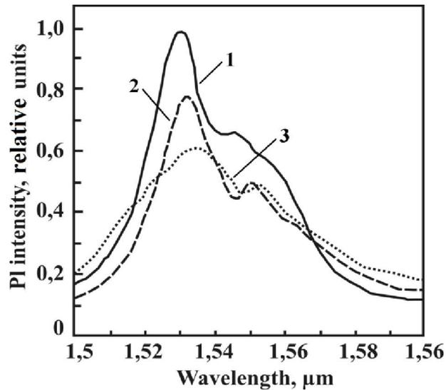
Fig. 4. Spectral characteristic of a film ( $\text{Er}_2\text{O}_3 - \text{SiO}_x - \text{Al}_2\text{O}_3$ ) on the fragment of optical fiber in heating
