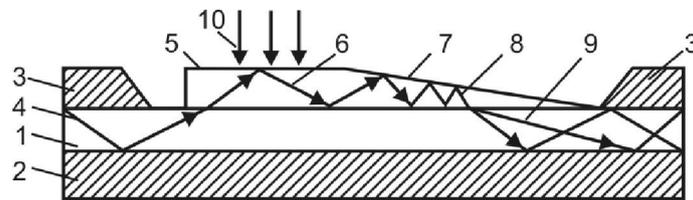
**Fig. 2.** A thin-film planar lightguide with the narrowed edge, generated on a fragment of a core of an optical fiber
