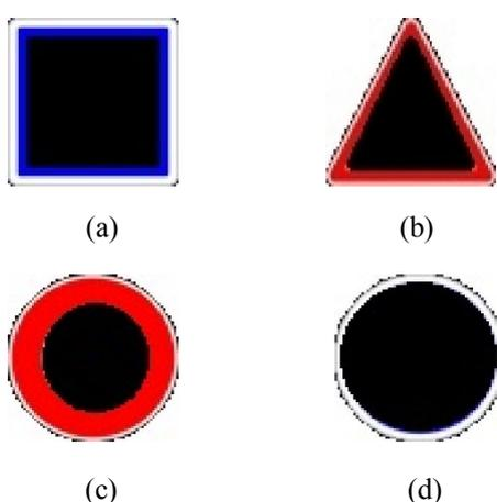
**Fig. 5. The signs models, (a) indication, (b) warning (c) Prohibition (d) obligation**
