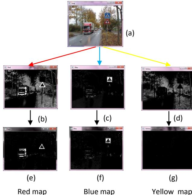
**Fig. 1.** Effect of the proposed filtering, (a) original image RGB, (b) (c) (d) segmented images before filtering; (e) (f) (g) after filtering segmented images
