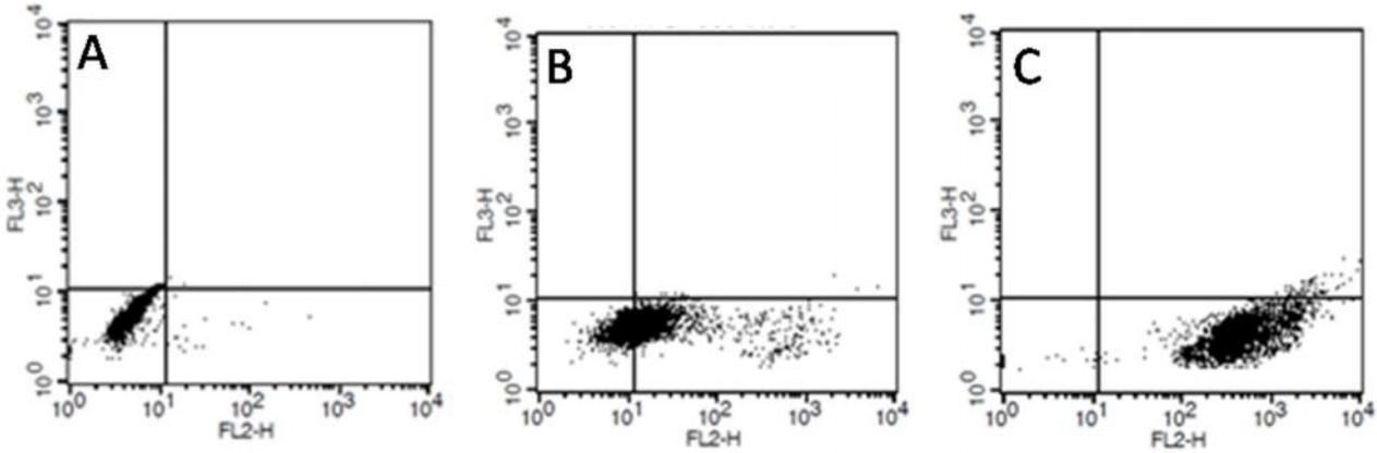
**Fig. 5. Improvement of *Dunaliella sp.* staining efficiency using DMSO. This strain has been isolated from saline in North Morocco, and experiment was carried out in our laboratory. A: microalgae sample without staining, parameter settings are adjusted to place population in upper left area. B: Nile red addition and incubation at 37°C during 10 min. C: NR staining improvement after addition of DMSO 20% simultaneously to NR addition. Data not published**
