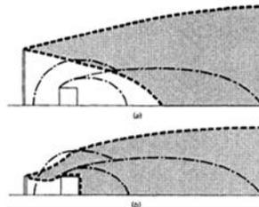
Figure 8 separation effects in smoke column dispersion
