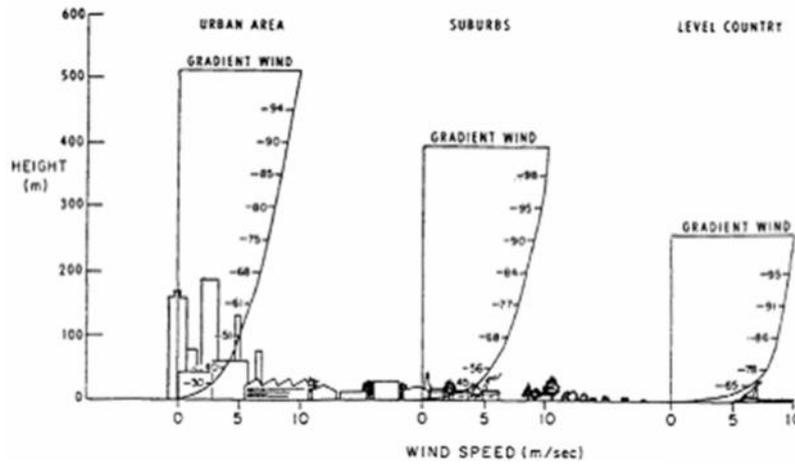
Figure 2 Effect of surface roughness on the velocity
