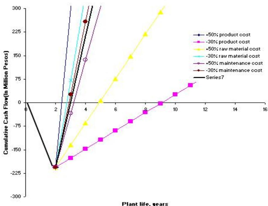
Fig. 1.7 Sensitivity analysis for cumulative cash flow
