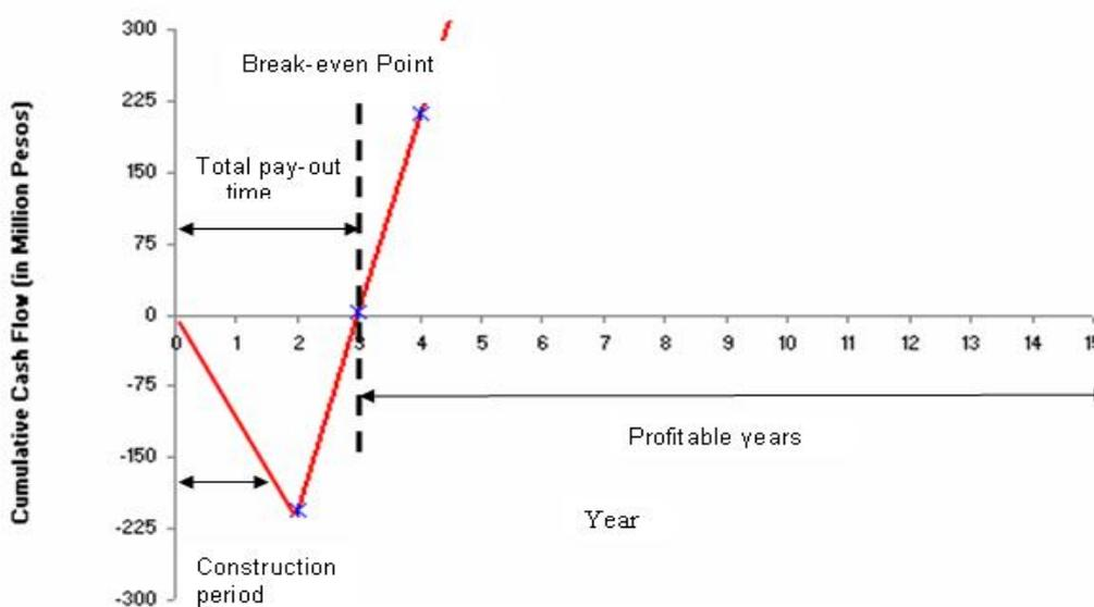
Fig. 1.6 The cash flow diagram
