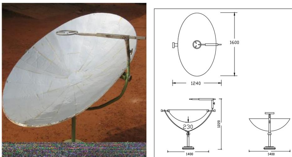
**Fig 1: Fibre reinforced plastic solar energy cooker**
