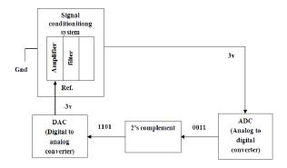
Fig. 6. offset calibration block diagram
