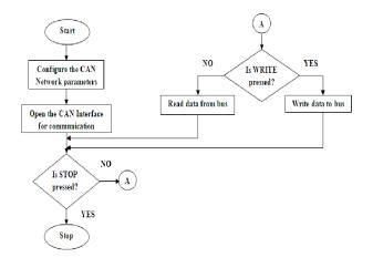
Fig. 5. LabVIEW CAN program flow
