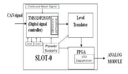
Fig. 3. New slot-0 block diagram
