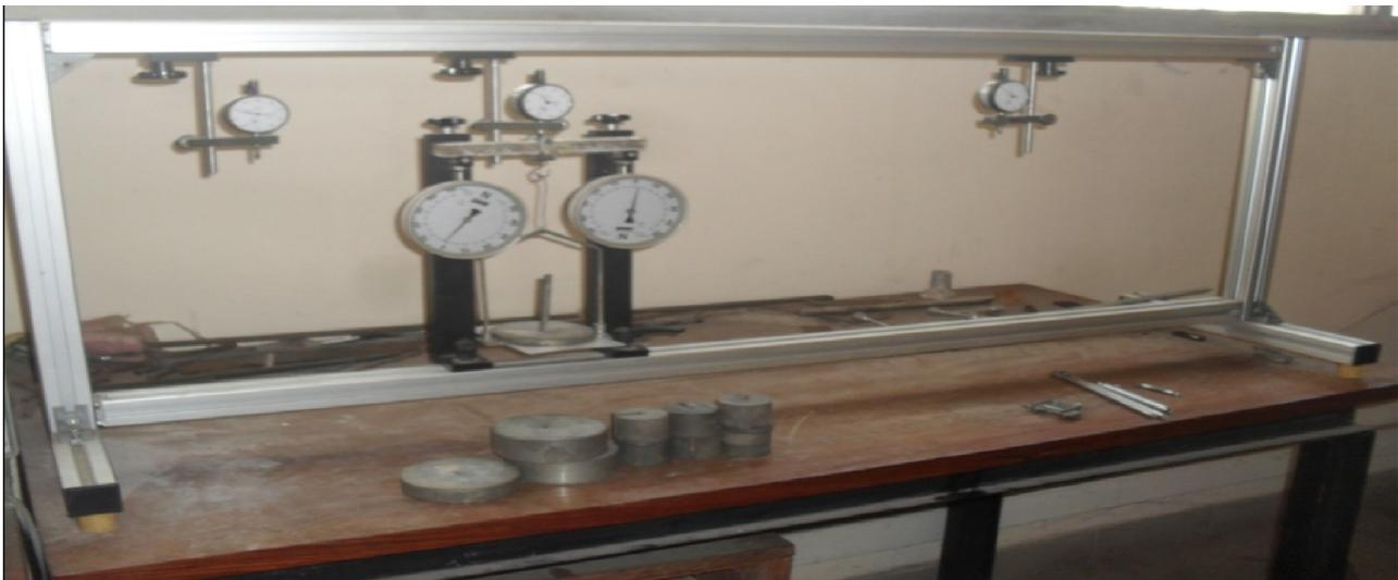
*Fig.1: testing machine "3 point" bending*
