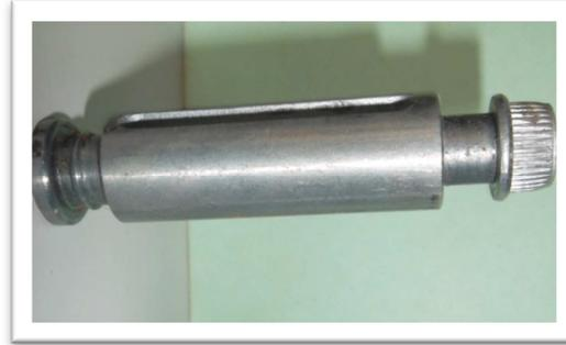
*Plate 2: Machined specimen for wear test*
