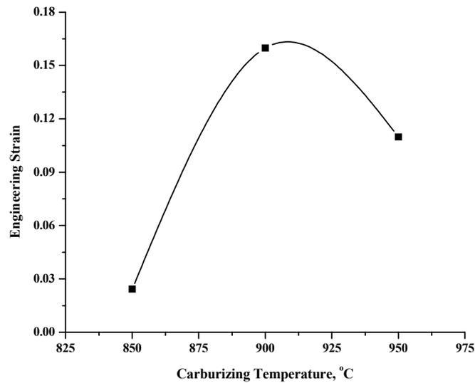
**Figure (4): The effect of carburizing temperature on the engineering strain of the samples**
