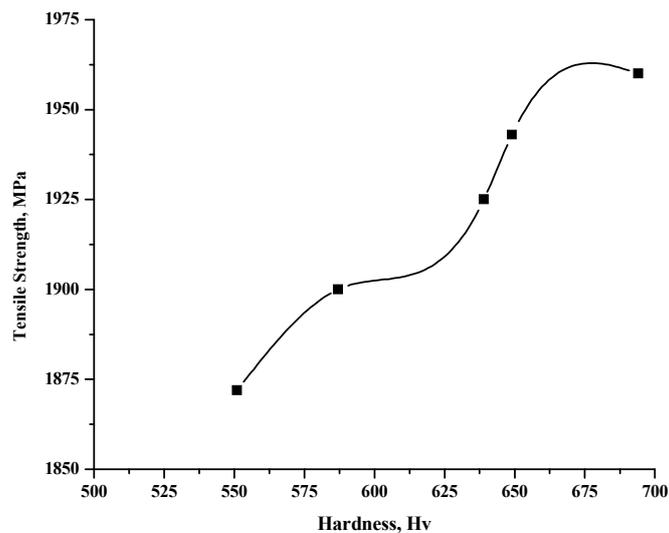
*Figure (8): Variation of tensile strength with hardness for carburization temperature.*
