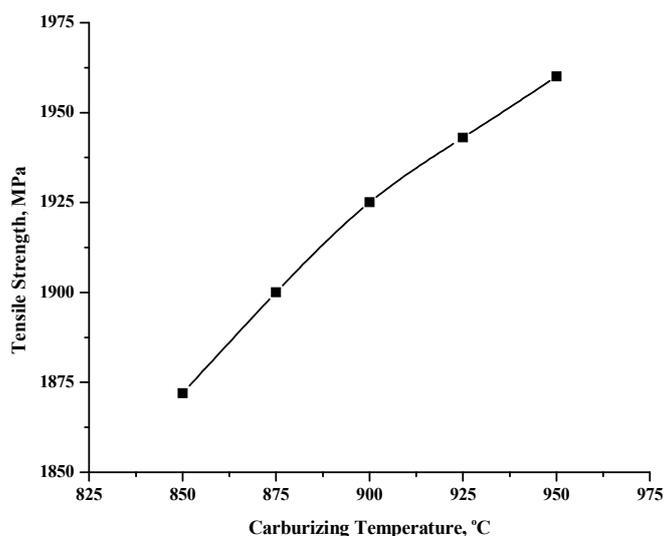
Figure (2): Variation of tensile strength with carburization temperature.
