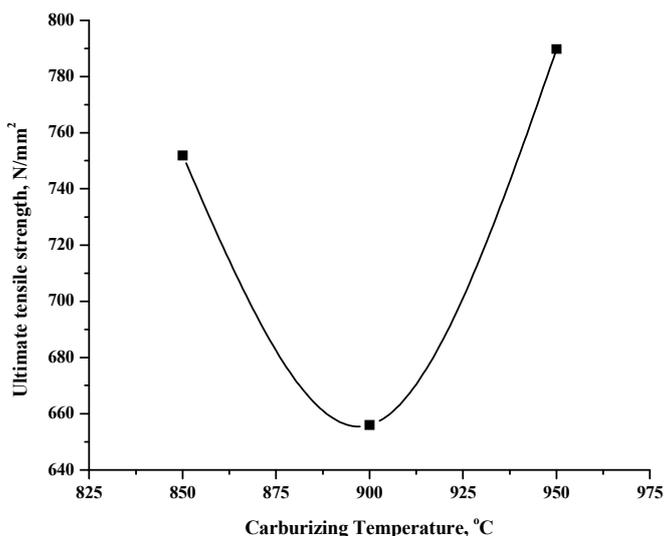
Figure (3): The effect of carburizing temperature on the ultimate tensile strength of the samples
