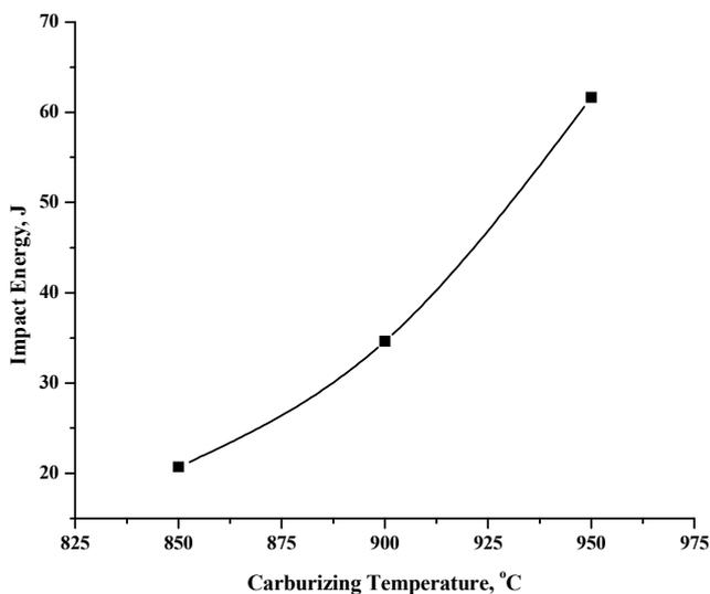
Figure (6): The effect of carburizing temperature on the impact energy of the samples.
