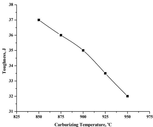
Figure (7): Variation of toughness with carburization temperature
