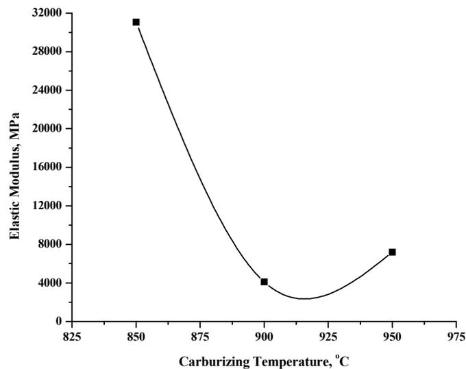
**Figure (5): The effect of carburizing temperature on the Young's modulus of elasticity of the samples**
