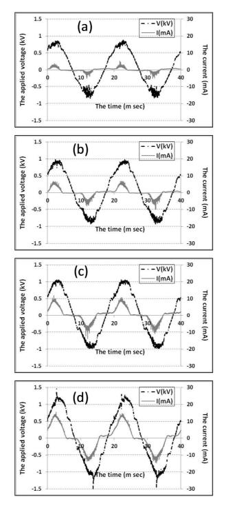
Fig. 2 I-V wave forms at different applied voltage
