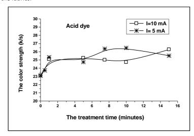
Fig. 7 Effect of air plasma treatment time on the colour strength of wool/polyamide fabric printed with acid dye.
