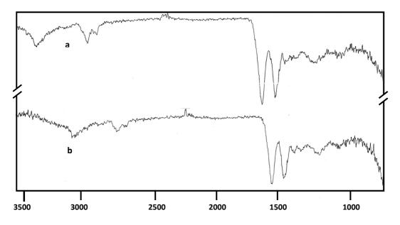
Fig.6 IR spectra of woo/polyamide fabric, (a) untreated, (b) air plasma treated fabric for 10 min., at 10 mA.
