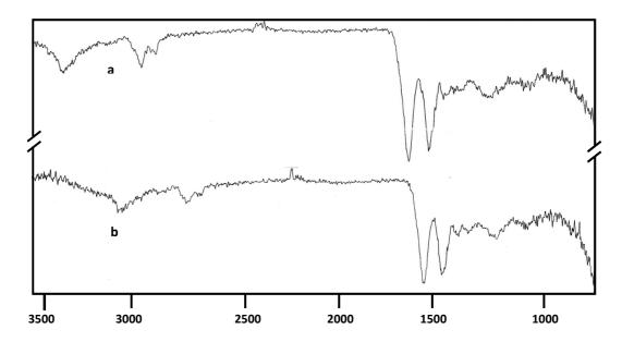
Fig. 6 IR spectra of woo/polyamide fabric, (a) untreated, (b) air plasma treated fabric for 10 min., at 10 mA.
