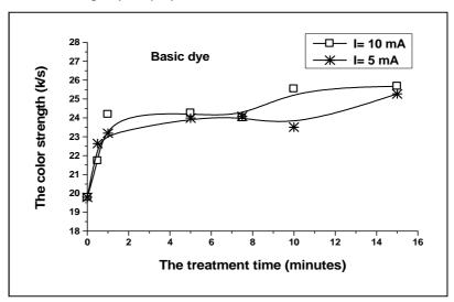
Fig.8 Effect of air plasma treatment time on the colour strength of wool/polyamide fabric printed with basic dye.
