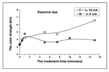
*Fig.9 Effect of air plasma treatment time on the colour strength of wool/polyamide fabric printed with reactive dye.*
