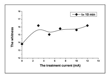
Fig.4 Effect of air plasma treatment on whiteness index of wool/polyamide fabric as a function of discharge current.
