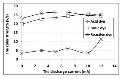
Fig.10 Effect of plasma discharge current on the colour strength of wool/polyamide fabric printed with acid, basic and reactive dyes.
