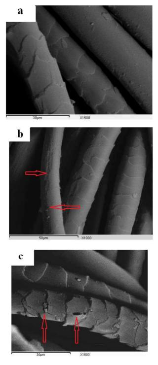
Fig.5 SEM pictures of (a) untreated, (b, c) air plasma treated wool/polyamide samples at 10 mA for 10 min.
