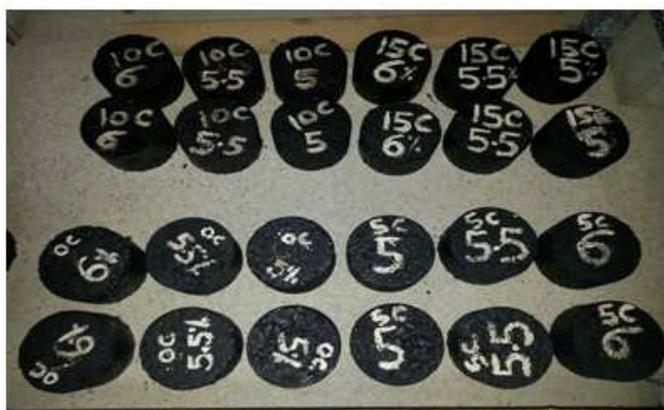
Fig. 1. Marshall Specimens casted for the study.
