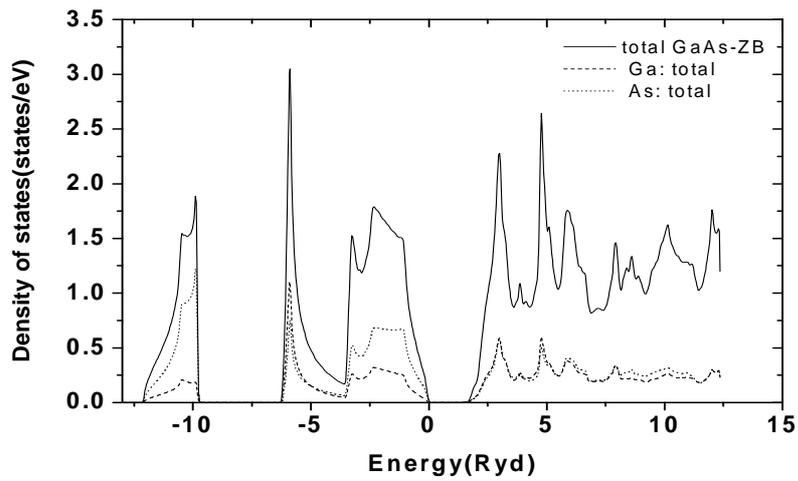
Fig. 7a. Total DOS of GaAs-ZB structure.
