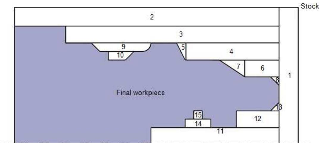
Fig. 16. Chronological order to remove machining features from the stock
