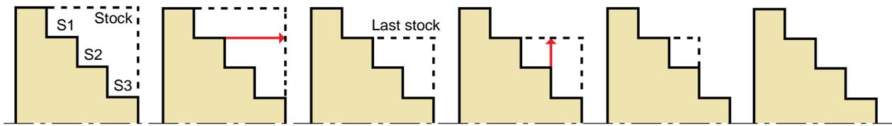
Fig. 12. Generation of features by extending their material surfaces until the stock surfaces
