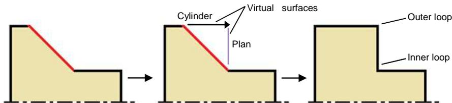
Fig. 6. Ring addition for a taper
