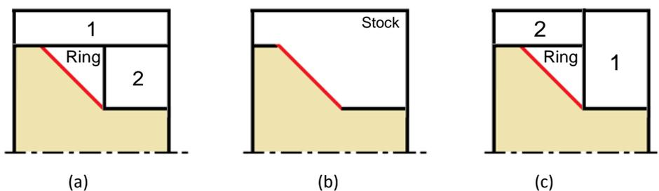
Fig. 14. Association of the ring to the taper with enveloping features
