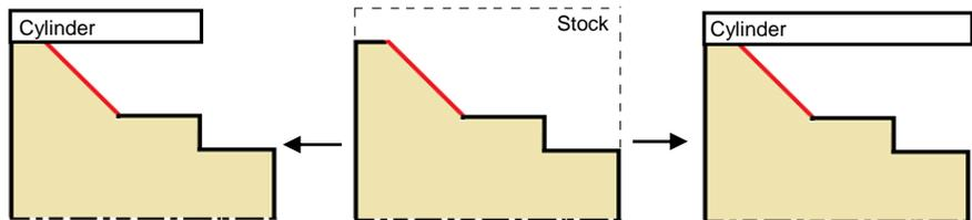
Fig. 4. Cylinder created from a taper (Ersan, 2005)
