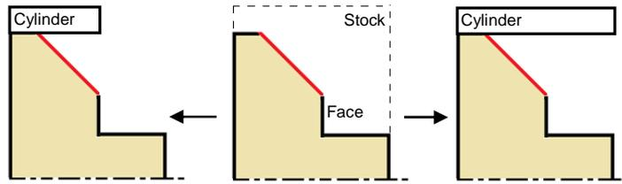
Fig. 7. Cylinder created from a chamfer (Ersan, 2005)
