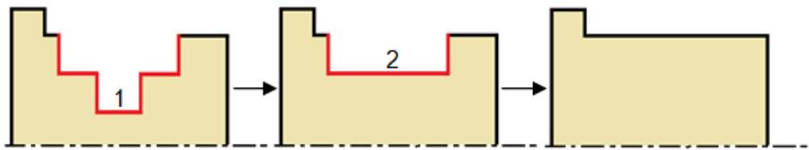
Fig. 3. Rings addition for nested grooves
