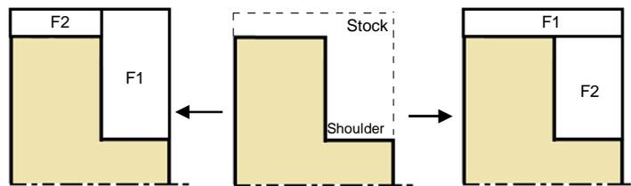
Fig. 8. Interacting features resulting after adding a ring to the chamfer
