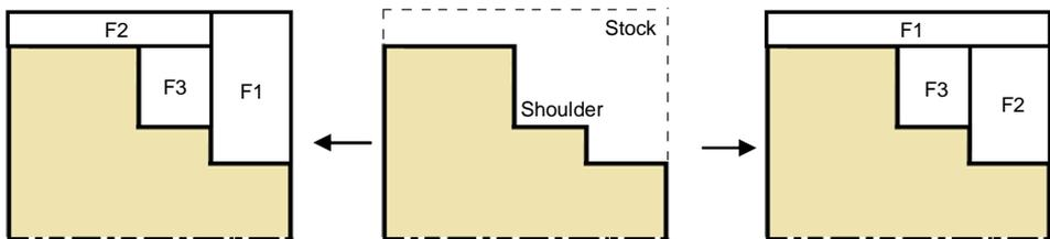
Fig. 5. Some interacting features resulting after adding a ring to the taper
