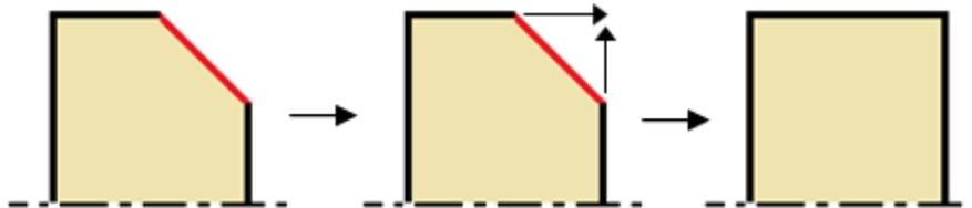
Fig. 9. Ring addition for a chamfer
