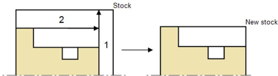
Fig. 10. Suppression of the face and the cylinder features from the stock
